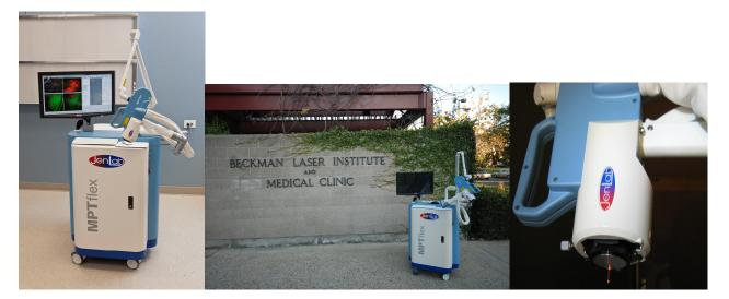
Fig. 1. Images of the Prism-Award winning device multiphoton tomograph MPTflex<sup>TM</sup>. The scan head consists of a 3D scanning module, the focusing optics, two detectors for fluorescence and SHG imaging, and a 1.7 mm thick microendoscope. Photo (left) taken by Paul Kennedy.
