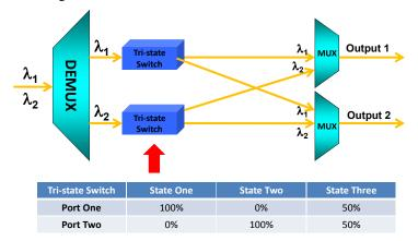
Fig.5 Tri-state example for reconfigurable router
