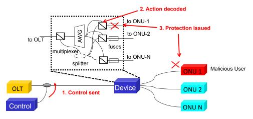
Fig.4 Node architecture of optical countermeasure
