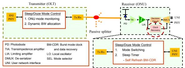
Fig.9 Proposed energy conserving TDM-PON architecture using sleep mode ONU with fast wake-up capability
