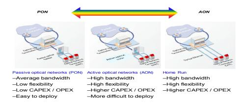
Fig.1 Optical Access Network Technology
