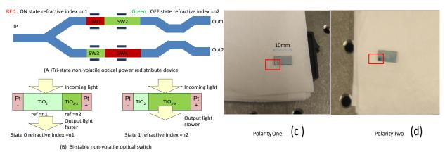
Fig.7 transition metal oxide based switch (a),(b) MZI based tri-state switch, (c)(d) non-volatile change of optical property.
