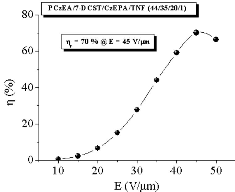
Figure3. High diffraction efficiency for p-polarized beam
