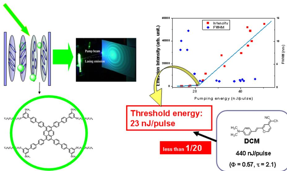
By using new pyrene and anthracene derivatives that have both high luminous efficiency and high solubility in CLCs, we have attained lower lasing thresholds in dye-doped DFB CLC lasers. The threshold values were decreased to one twentieth that of DCM.
