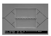
Figure 5. SEM image of a microfabricated array of funnels for bacteria.
