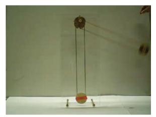
Figure 2. Snap-shot of the motion of 2 pendula coupled by a linear torsional spring. Energy stays trapped in the moving pendula.
