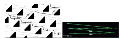
Figure 9. Using double-broken sym- Figure 10. Realization of the ratchmetry to obtain true ratcheting mo- eting motion in symmetrical flow. tion at low Re: basic scheme.
