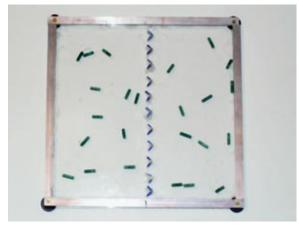
Figure 3. The constructed funnel line before shaking. The aluminum "molecules" are painted green.
