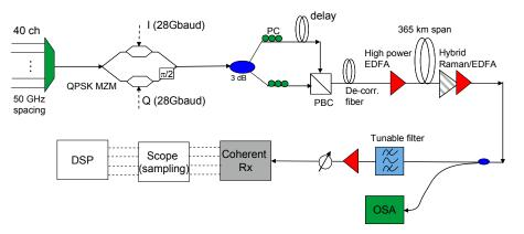
Figure 4: Experimental set-up for 365 km unrepeatered span transmission system experiment.
