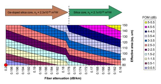
Figure 1: Fiber FOM as a function of attenuation and effective area for 75 km span length. Red circle represents parameters of reference fiber.
