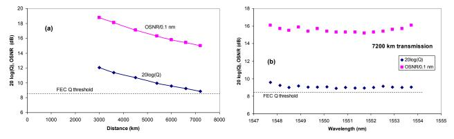
Figure 9: (a) BER and OSNR vs. transmission distance for 1550.92 nm channel. (b) OSNR and Q values for all 16 channels after 7200 km transmission.
