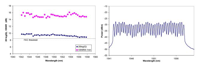
Figure 15: (a) 20log(Q) and OSNR/0.1nm for all 40 channels at 10,200 km distance. (b) Optical spectrum at 10,200 km.
