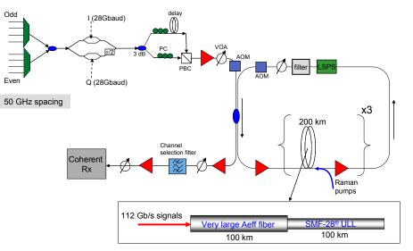
Figure 10: Experimental set-up for re-circulating loop experiments with 200 km fiber spans.
