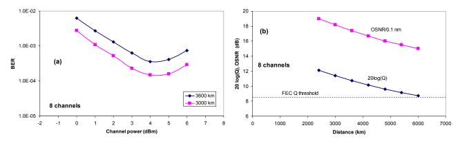
Figure 11: 8 channel transmission data for 1548.51 nm channel. (a) BER vs. channel power, (b) Q and OSNR vs. distance.
