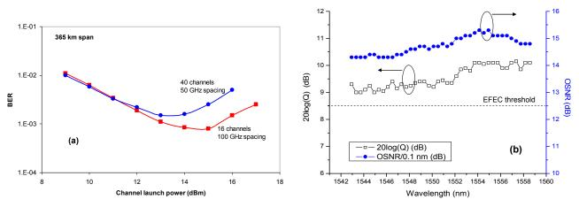
Figure 6: (a) BER vs. channel launch power for 40 channel, 50 GHz system, and 16 channel, 100 GHz system. (b) OSNR (0.1 nm noise bandwidth) and 20log(Q) values of all 40 channels after transmission over 365 km unrepeatered span.
