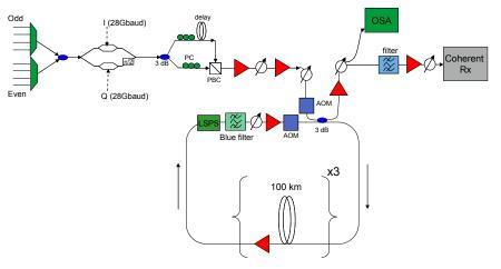
Figure 7: Experimental set-up for 16 channel, 100 km span, EDFA-only, re-circulating loop experiments.
