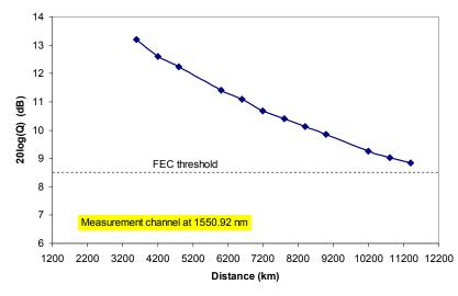
Figure 14: 20log(Q) vs. transmission distance for 1550.92 nm channel in all-Raman amplified system using Vascade<sup>®</sup> EX2000 optical fiber.
