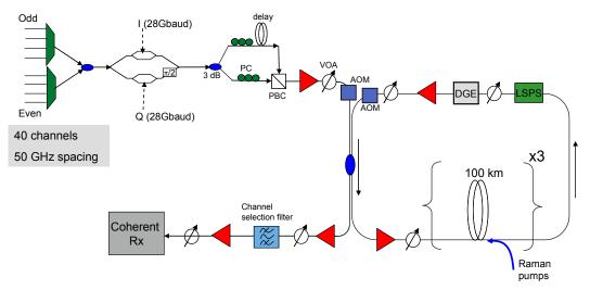
Figure 13: Experimental configuration for 40 channel all-Raman amplified transmission system.
