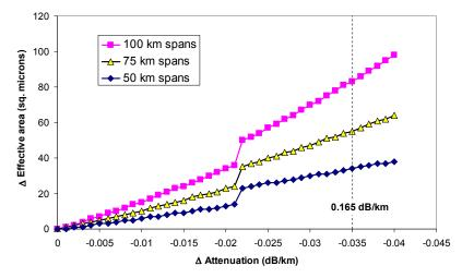
Figure 2: Relative impacts of decreasing fiber attenuation and increasing fiber effective area with respect to the reference fiber, for system span lengths of 50, 75, and 100 km.
