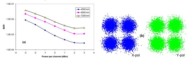
Figure 8: (a) BER vs. channel power for 1550.92 nm channel at 3 different transmission distances. (b) Typical PM-QPSK constellation diagram after 7200 km transmission.
