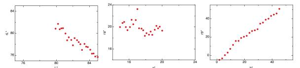
Figure 8: Plotting the colors sent to the printer vs. those actually printed reveal the problems of this printer in the range of interest from (80, 15, 2) to (85, 20, 45).
