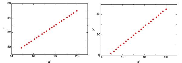
Figure 5:  $L^*a^*$  respectively  $a^*b^*$  plot of the uniform color scale in CIE 1976 ( $L^*a^*b^*$ ) from (80, 15, 2) to (85, 20, 45) in steps of 2  $\Delta E$ . The non-uniformities are due to rounding the coordinates to one decimal digit.
