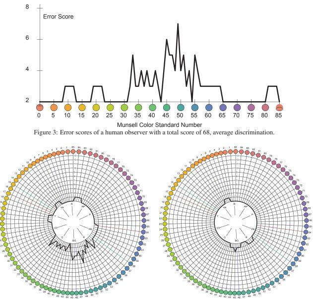
Figure 4: Left: Same error scores as in Fig. 3, but plotted in a polar diagram; there is no diametrical symmetry, suggesting the observer has normal color vision. Right: diagram of an observer with total score 16, superior discrimination.
