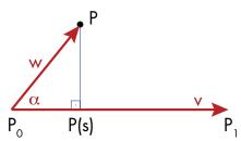
Figure 10: Introducing the two vectors v, w the parameter s can be calculated as the ratio of two scalar products.
