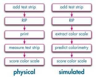
Figure 12: Workflow in physical respectively simulation mode.
