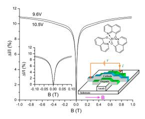
Figure 1. Typical magnetic-field effect traces for Alq<sub>3</sub> OMAR devices. The insets show the OMAR traces plotted over a smaller magnetic-field range, the Alq<sub>3</sub> molecular structure and the schematic OMAR device structure.
