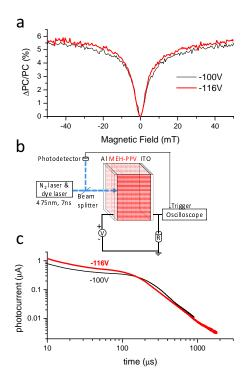
Figure 2. a) Magnetic field effect on the continuous wave photocurrent vs. magnetic field for two different reverse biases. b) Schematic drawing of the photocarrier time of flight setup. c) Time-resolved photocurrent for two different reverse biases.
