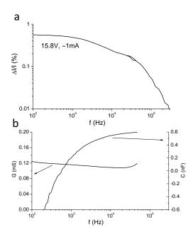
Figure 4. a) Magnetic field response  $\Delta I/I(0)$ , of the device current of an Alq<sub>3</sub> OMAR device to an applied AC magnetic field of frequency f. b) Frequency-dependent conductance G and capacitance C at 15V.
