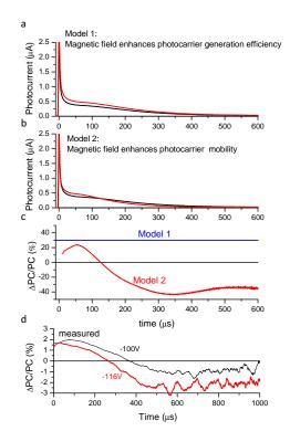
Figure 3. Magnetic field effect on the time-resolved photocurrent. a) Hypothesized scenario that the magnetic field affects the carrier generation efficiency (referred to as Model 1), b) Hypothesized scenario that the magnetic field affects carrier mobility (Model 2). c) Simulated magnetic field effects on the time-resolved photocurrent based on Model 1 and Model 2. d) Measured traces for two different reverse biases.
