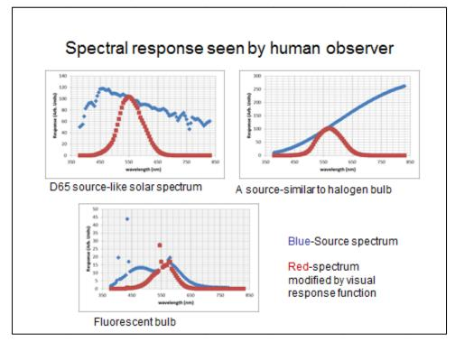
Figure 2. Example of the spectral response of a human observer viewing three different standard sources.
