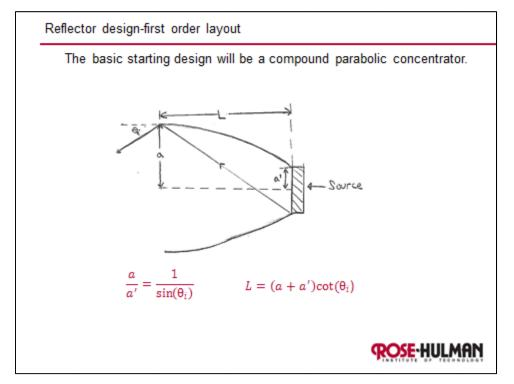
Figure 4. Example slide from a student's design evaluation report illustrating the basic concept of a CPC as the starting point of the design of a luminaire.
