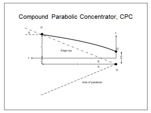
Figure 3. Drawing illustrating the geometry used in defining edge rays and angles a compound parabolic concentrator.
