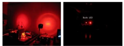
Figure 2 - (Left) Light output for bulb (left) versus LED (right). (Right) Visibility of bulb (left) versus LED (right) at 30 ft.
