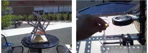
Figure 5 - (left) the completed solar tracker/collector. (right) close-up of lens, fiber collimator and output from the end of the fiber. Not visible is an IR filter located above the lens.
