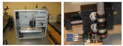
Figure 1 - (Left) Prototype LED enclosure. (Right) High powered LED mounted for x-y positioning.
