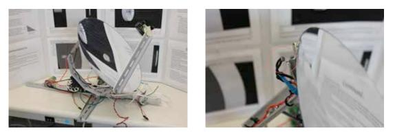
Figure 6 – Revised version of the solar tracker/collector using a lightweight Cassegrain mirror system. Left: Mirror assembly with motor to the left. Right: Light sensors are mounted below the rim of the mirror on opposite sides.
