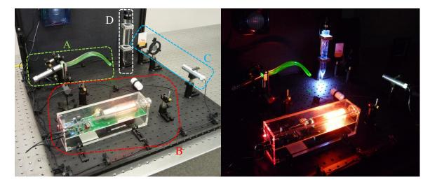
**Figure 4.** Fiber optics set-up showing total internal reflection (A), wireless communication (B), transmittance of materials (C) and a fiber optics pre-form (D).
