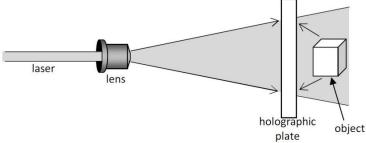
Figure 1. Schematic representation of the creation of reflection holograms
