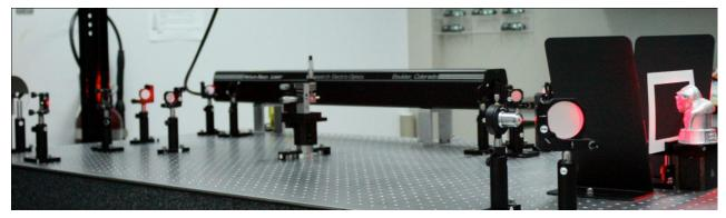
**Figure 2.** The 35mW He-Ne laser beam is split, filtered and spread out to uniformly illuminate the object in this demonstration of how holograms are exposed. The black panels on the right block light from sideways illumination that could cause interference in the holographic plate.
