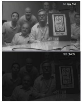
Fig. 56 Images collected in a completely dark room. The only illumination is from a 940 nm LED. The upper image is the XQE sensor and the lower is a standard CMOS sensor. Both sensors have 380  $\times$  240 resolution and 11.2  $\mu$ m pixels. The integration time for both is 16 msec.
