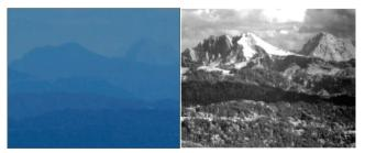
Fig. 6. Scene of the Swiss alps taken at a range of 37 km during a sunny day. Visible is shown on the left and SWIR on the right.
