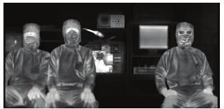
Fig. 44 Image taken with a  $2000 \times 1000$  uncooled array fabricated with SOI technology. NE $\Delta$ T for this 15  $\mu$ m pixel array was 65 mK.
