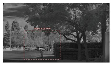
Fig. 13. Daytime imagery taken in integrate while read (IWR) mode from a  $1920 \times 1080$ , 15  $\mu$ m pixel pitch, low noise InGaAs SWIR sensor. The field of view of a  $640 \times 512$ , 15  $\mu$ m sensor is shown by the dashed box outline.
