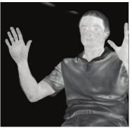
Type II superlattice Fig. 17 Image taken with a 1024×1024 energy transitions LWIR Type II superlattice detector.
