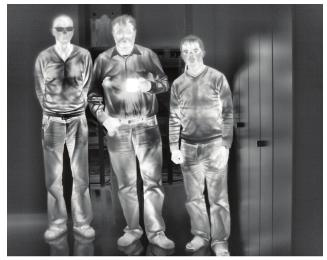
Fig. 25 Image taken with an LWIR HgCdTe FPA having a 1280  $\times$  1024 format and 15  $\mu$ m pixels.
