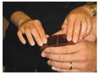
Braille screen fabricated on a plastic sheet.
