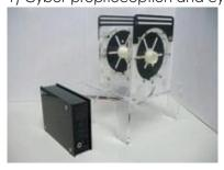
Like natural muscles, DE-based artificial muscles can now provide in real time both positional feedback (cyber-proprioception) and condition-monitoring information (cyber-pain). These capabilities, essential for the control and performance of soft machines, will be demonstrated using the lab's Self-Sensing Unit coupled to a DE actuator.
