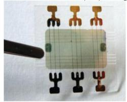
Array of 72 devices on a 2×2 cm<sup>2</sup> chips
