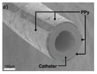
A catheter is coated with polypyrrole, and patterned to enable tip deflection. This is intended to enable navigation and imaging within the neuro-vascular system.
