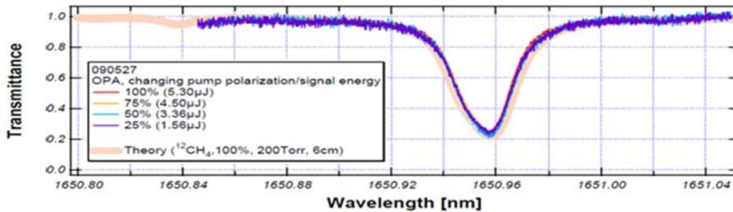
Fig. 3. Scan of Methane lines at 1650.96 nm using the GSFC OPA system.
