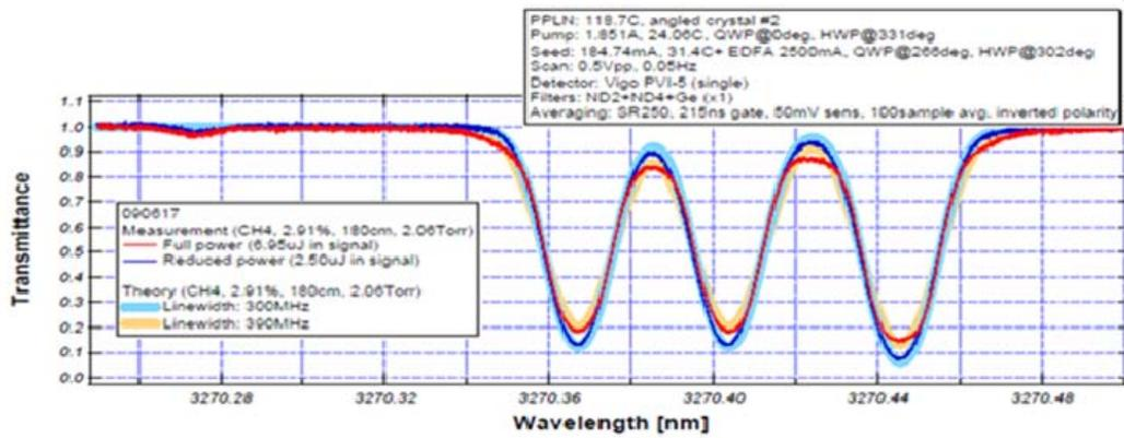
Fig. 2. Scan of Methane lines at 3270.40 nm using the GSFC OPG system.
