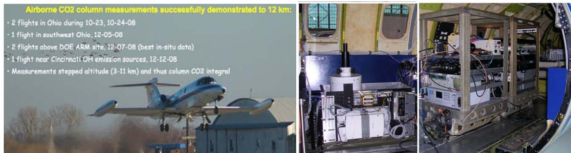
Fig. 1 (left) The NASA Glenn Lear-25 carrying our airborne precursor CO<sub>2</sub> lidar instrument during December 2008. (right) Photograph of the interior of the Lear aircraft showing the fall 2008 version of the instrument, with (left to right) the receiver telescope assembly, the laser and electro-optics rack and the electronics/computer rack.
