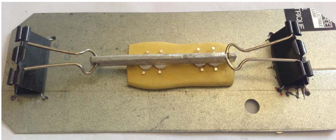
Fig. 5. Soldering rig for easy soldering of the piezoelectric element leads. The paper clips and bar hold down the LEDs. The yellow in the center is ordinary craft silicone that has cured.
