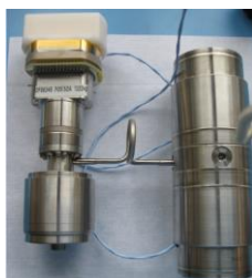
Figure 4: SOFRADIR space Dewar and cooler assembly for MARS and SATURN detectors
