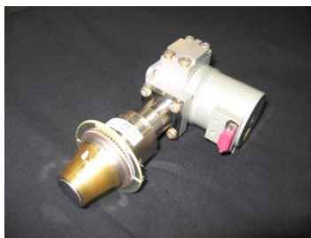
Figure 2: MARS MW IDDCA integrated in NOMAD instrument
