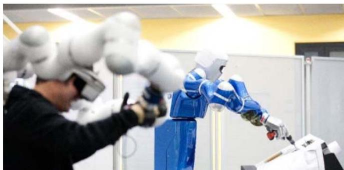
Figure 1: Operator using HUG to control SpaceJustin
