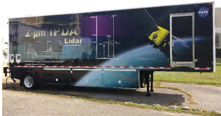
Fig. 6. Picture of the mobile lidar laboratory. Located at NASA LaRC, the laboratory is used for IPDA instrument integration and horizontal and vertical pointed ground testing, as well as future field deployment.
