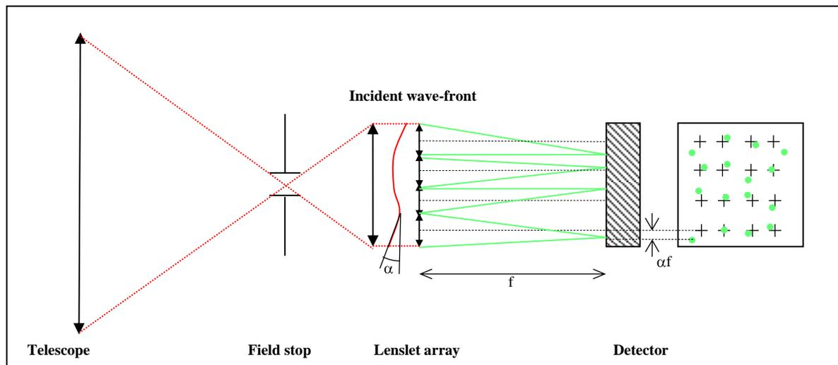
Figure 1 Principle of the Shack Hartmann wave-front sensor
