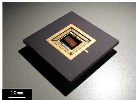
Figure 1. 64 x 32 micromirror array with high fill factor in the vertical direction providing long slits. Each mirror measures 200 x 100  $\mu\text{m}^2$ . Two wafer level bonding steps are required to process these arrays.
