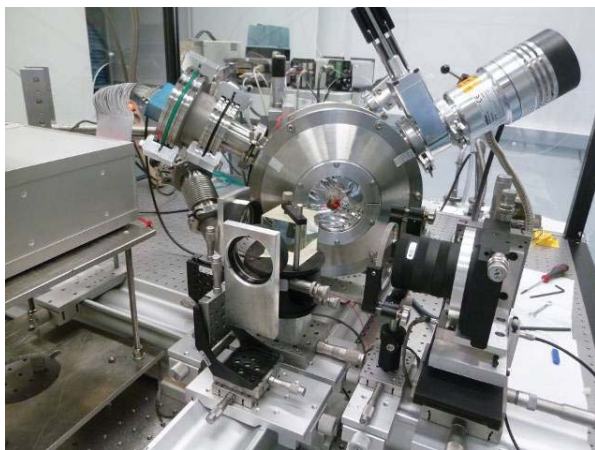
Figure 2. Cryogenic chamber installed on our interferometric setup. MMA with 64 x 32 micromirrors is integrated (100 x 200 \mu\text{m}^2 micromirrors).
