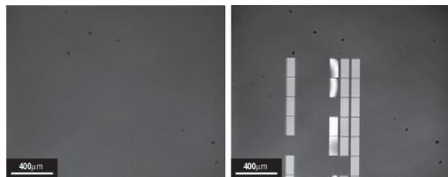
Figure 3. Interferometric observations of the lines of micromirrors during the cryogenic experiment at 162K: micromirrors at rest (OFF state) and in ON state when 148V is applied. Mirrors are tilted by 24°.
