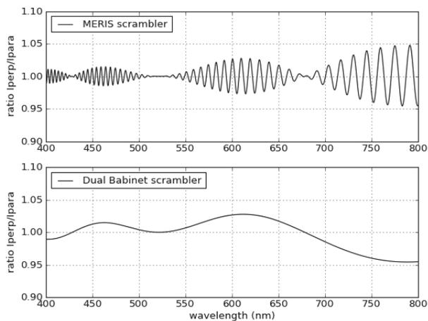
Figure 5. (top) Simulated ratio of measured intensities behind the MERIS scrambling window assembly (SWA) placed between crossed and parallel polarizers. No spectral smoothing is used, the simulated scrambler has a perfect rectangular pupil 20\*40mm and wedge angles of 8mrad. (bottom) The simulation is repeated for an equivalent Dual Babinet with a wedge angle 4mrad : we recover the envelope of the MERIS oscillations.
