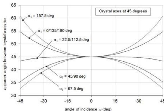
Figure 7. Deviation between the apparent angle  $\Delta\alpha$  and true angle  $\alpha_2 - \alpha_1$  between the crystal axes at the W2/W3 interface in a Dual Babinet scrambler.
