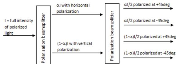
Figure 2. Working principle of a fully depolarizing scrambler, described with polarization beamsplitters (PBS). The full intensity after two PBS is 1/2 polarized at +45 degrees, and 1/2 polarized at -45 degrees.
