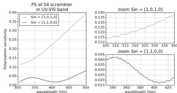
Figure 6. Calculated polarization sensitivity for the scrambler design of Sentinel-4 phase A. The instrument is replaced with a linear polarizer having the worst case orientation. Left : PS curves for polarization states along the axes of strong (black) and weak (gray) depolarization. Right : zoom showing the spectral oscillations in the PS curves.
