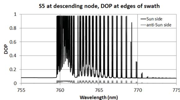
Figure 1. Spectral variations of the degree of polarization (DOP) observed by Sentinel-5 at its descending node, on both edges of the instrument swath. A mid-latitude summer AFGL profile is assumed, with a layer of continental aerosol with optical depth 0.2 located between 900 and 700 hPa, and a ground albedo of about 0.35 representative for healthy vegetation.
