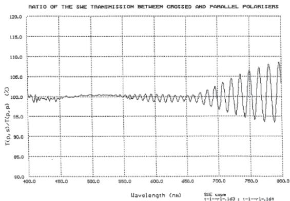
Figure 4. Ratio of measured intensities behind the MERIS scrambling window assembly (SWA) placed between crossed and parallel polarizers [8]. In this experimental result, the oscillations are smoothed by the measurement bandwidth of 5nm and then almost disappear around 500nm. The pupil is 20\*40mm with 2 rounded corners.
