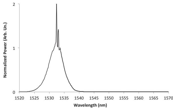
Figure 8. Self-lasing observation from over pumped source
