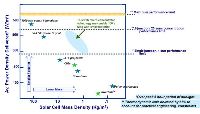
*Figure 4.* A plot of commercially available solar technology shows a trade-off between power density and mass density. It is envisioned that combining PIC technology and micro-concentration will enable PV performance that achieves unprecedented power-per-mass (blue oval) within a small footprint. The goal is to exploit the economies of scale for mass produced solar PV PICs and micro-optics to enable lower performance per cost than conventional PV panels may achieve.
