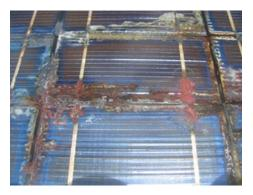
Figure 5: Corrosion of cell metallization from Arizona
