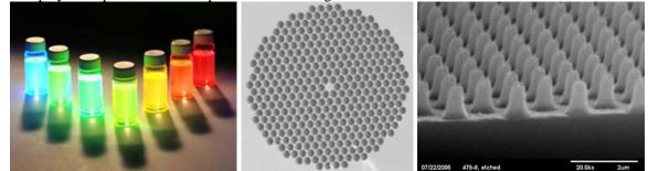
Fig. 1. Examples of nanophotonic materials and devices. These include quantum dots solutions (left), holey fibers (center), and diffractive sub-wavelength structures (right) designed and fabricated by the author.
