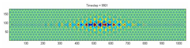
Fig. 3. Wave propagation in a slab photonic crystal waveguide. This example illustrates the concepts of optical waveguiding, light localization, and the process of coherent scattering in a photonic nanostructure.
