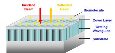
Fig. 5. Resonant reflecting structure used to illustrate the research and development of a new biosensing platform for protein detection using nanophotonic structures.
