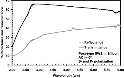
Fig. 4. Reflectance and transmittance spectra for a two-dimensional SWS structure designed for broadband antireflection (AR) operation in the  $2 - 6 \mu m$  MWIR wavelength range.
