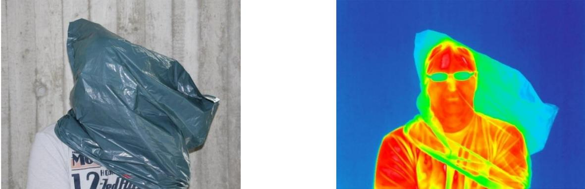
Figure 8: Plastic bags are partially transparent to IR radiation (which may also be quantified using IR spectroscopy)
