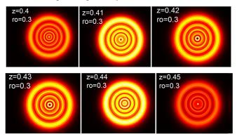
Fig.1 Fresnel diffraction patterns for a circular aperture.
