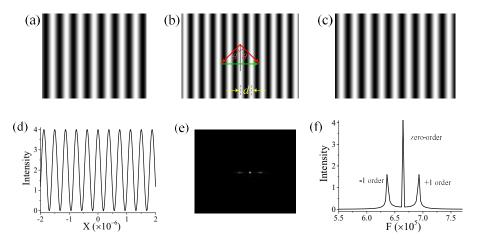
Fig.3 (a)-(c) Interferograms with different parameters; (d) the intensity distribution, (e) 2D and (f)1D frequency spectrum of (b).
