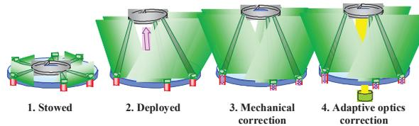
Fig. 1: Deployment stages
