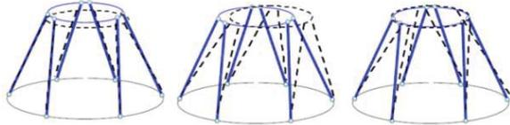
Fig. 4: Natural mode shapes: pumping, tilt and torsion.
