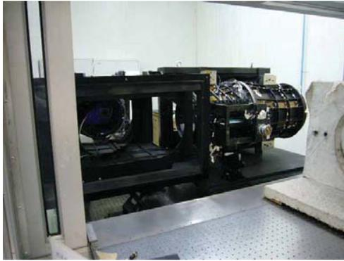
Figure 5. The Setup of the Optical MTF Test
