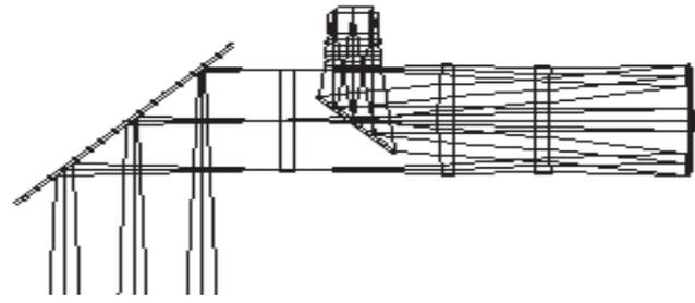
Figure 2. Optical system of PMS camera
