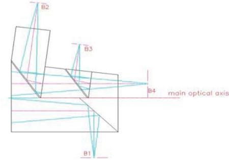
Figure 3. Light splitted in the Prism
