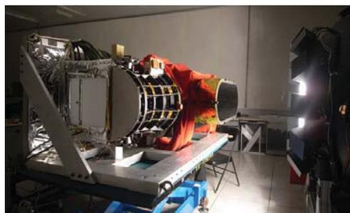
Figure 10. Integral Sphere Test
