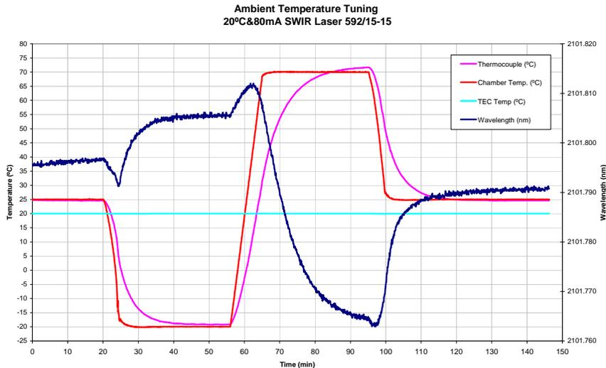
**Figure 3.** SWIR wavelength variation (dark blue line; right axis) with ambient temperature cycling for a laser diode TEC controlled temperature of 20 $^{\circ}\text{C}$  (light blue line). The red line is the actual chamber temperature and the purple line is the laser package temperature measured with an additional thermocouple.
