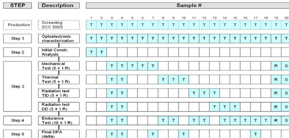
**Figure 1.** SWIR Laser test flow proposed for 20 samples. (T means sample to be Tested, R means Reference and S means Spare; the samples came from two different lots)
