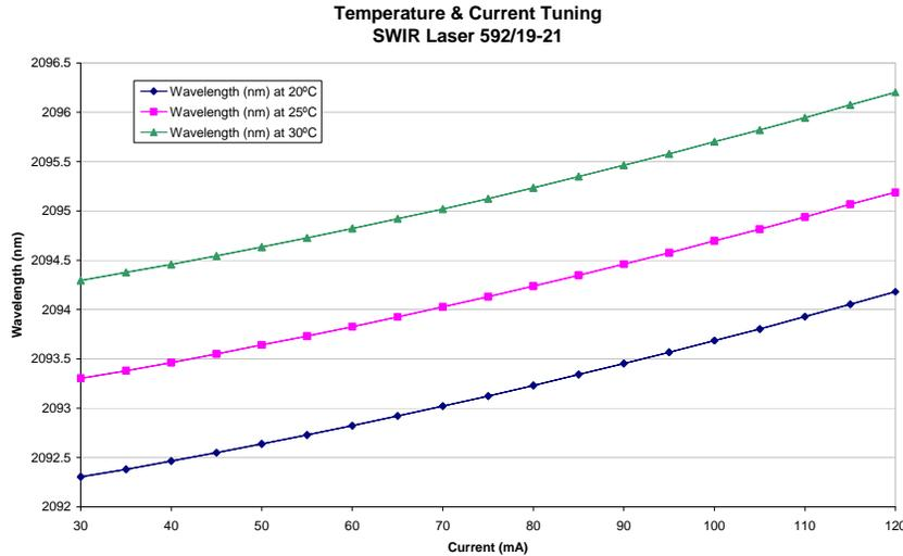
**Figure 2.** SWIR Laser temperature and current tunability
