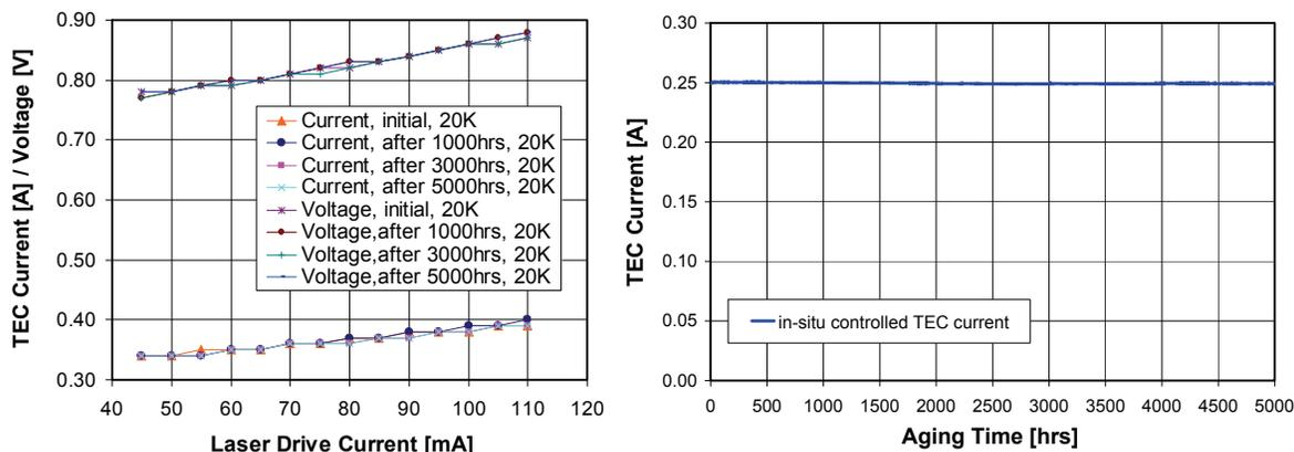
**Fig. 6.** TEC current and voltage at temperature difference of 20K vs. laser drive current (left diagram); in-situ monitoring of TEC current over aging, TEC temperature 40°C/case temperature 55°C (right diagram)
