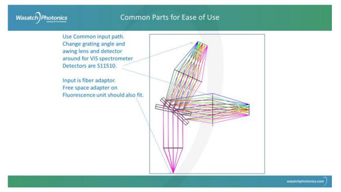
Figure 6 – Diagram of some common parts
