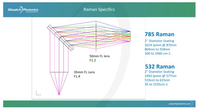
Figure 4 –Diagram of two different Raman sources with different gratings
