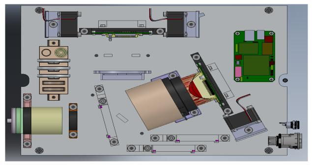
Figure 10 - Sand Box Top View of Raman Spectrometer
