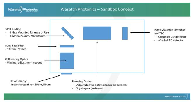
Figure 3 – Block Diagram of the Internal Components, with some having multiple options
