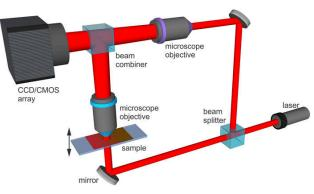
Figure 1. Diagram of the Mach-Zehnder microscope for off-axis digital holographic interferometry [1].
