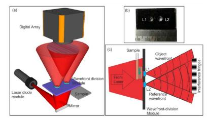
Figure 4. Diagram of the two lens wavefront division digital holographic microscope, b) wavefront division module housing the two lenses (L1 and L2), and c) diagram for the conversion of the incident source beam into an object and reference wavefront which interfere at the sensor [5].
