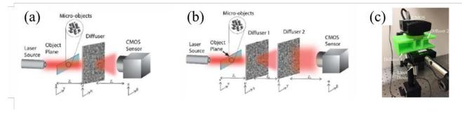
Figure 5. a) Single random phase encoding (SRPE) configuration b) double random phase encoding (DRPE) configuration, and c) experimental system used for both SRPE and DRPE experiments [19].
