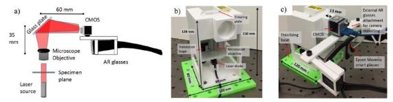
Figure 8. a) Proposed schematic for the augmented reality digital holographic prototype using a laser source, microscope objective, CMOS image sensor and the augmented reality (AR) device. b) The 3D-printed prototype, and c) the 3D-printed prototype with the AR glasses attached. The Epson Moverio smart glasses were used in the experiments [15].
