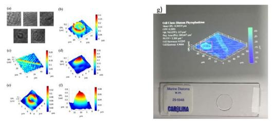
Figure 9. (a) Digital hologram of each of the five classes (from left to right: diatom phytoplankton, diatom pennate, navicula, selenastrum, and glass bead), and pseudocolor 3D rendering of the optical path length profile for (b) diatom phytoplankton, (c) diatom pennate, (d) navicula, (e) selenastrum, and (f) glass bead. g) Output as displayed to the augmented reality smart glasses, the source slide is visible in the background [15].
