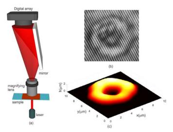
Figure 3. a) Diagram of the as Lloyd's mirror wavefront division, b) hologram of an RBC, c) reconstructed height profile of the RBC [1].
