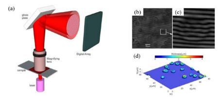
Figure 2. a) Schematic of the shearing microscope for off-axis digital holographic interferometry. b) Hologram of red blood cells (RBCs) recorded by the shearing interferometer, c) a zoomed in region for a single RBC showing fringes modulated by the cell, and d) thickness profiles of the RBCs calculated from the extracted phase profiles [1].
