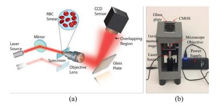
Figure 10. (a) Optical schematic of the overviewed shearing digital holographic microscope for cell analysis. (b) Image of the overviewed 3D-printed compact system [17].
