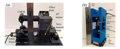
Figure 6. a) He-Ne based 3D-printed lateral shearing digital holographic microscope, and b) laser diode-based 3D-printed lateral shearing digital holographic microscope [14].
