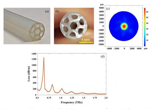
Figure 2. (a) Photograph and (b) cross-section of the hollow-core antiresonant fiber extruded from the metal 3D printed structured nozzle. (c) Simulated intensity profile of the fundamental mode at f = 0.7 THz. (d) Simulated transmission loss.
