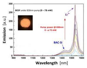
Figure 10. Spectral emission from one Bi/Er co-doped optical fiber draw from 3D printed silica preform.
