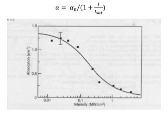
Figure 8; example of saturable absorption, transmission vs. intensity for CdSe QD glass
