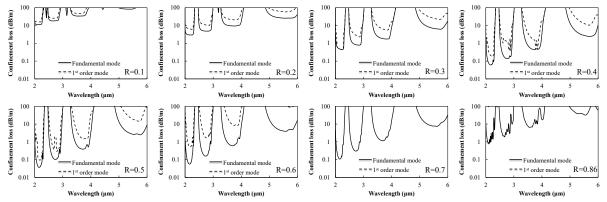
Figure 3. Calculated confinement loss of the fundamental mode and 1<sup>st</sup> order mode with different value of R (from 0.1 to 0.86).
