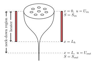
Figure 1: Schematic diagram of the neck-down region,  $0 \le x \le L$ , over which the initial cross-sectional area of the thread  $\chi^2_{in}$  reduces to that of the fibre  $\chi^2_{out}$  due to the large draw speed  $U_{out}$  relative to the feed speed  $U_{in}$ .
