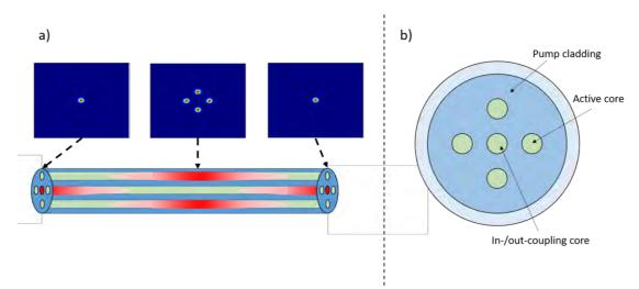
Figure 1. a) Schematic illustration of light propagation along the Talbot fiber. b) Cross-section of the proposed fiber design.
