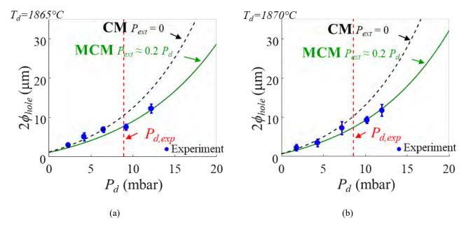
Figure 3. Experimental vs predicted results of the single capillary model (CM) and the modified single capillary model (MCM) at  $P_d = (0.1-16)$  mbar: (a)  $T_d = 1865$  °C and (b)  $T_d = 1870$  °C.
