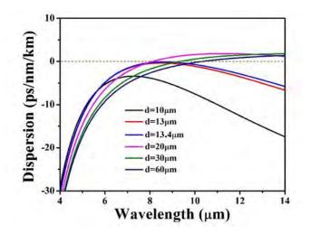
Figure 3. Calculated fundamental mode dispersion characteristic curves of Te-based ChG fibers with various core diameters.
