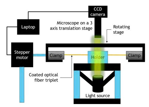
Figure 1: Scheme of the imaging system used for the sensor characterization
