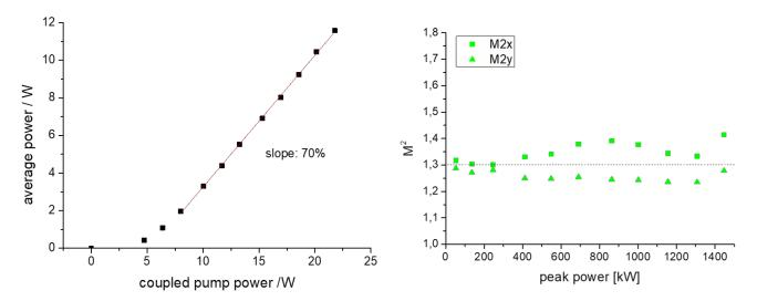
Figure 2. Slope efficiency and beam quality vs. peak power for a F-doped core fiber with 75 cm length.
