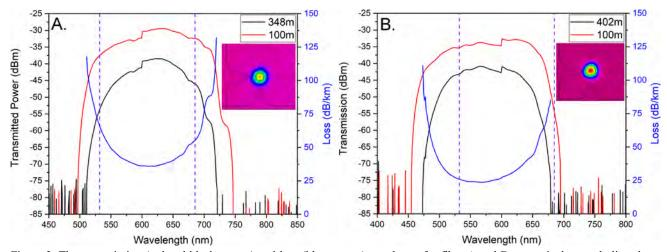
Figure 2. The transmission (red and black curves) and loss (blue curves) are shown for fiber A and B respectively, purple lines have been added to show the 532 and 683nm wavelengths as a guide to the eye. The obvious step feature at 600nm is due to the OSA switching gratings at that wavelength. Inset are beam profile images.
