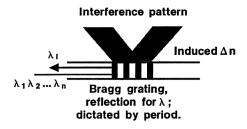
Figure 4; schematic of fiber Bragg grating, how it is fabricated, and how it functions in the fiber
