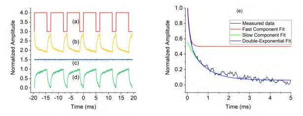
Fig. 4. (a) Input current into the laser diode. (b) Output signal with  $\cos(\Delta \phi') = -1$  (c)  $\cos(\Delta \phi') = 0$  (d)  $\cos(\Delta \phi') = 1$ .
