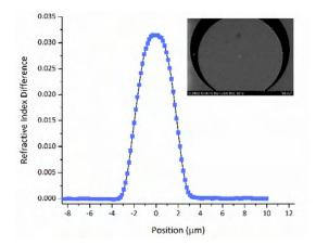
Figure 1: Refractive index profile with the 0 position being the center of the core with an image of the fiber inset.
