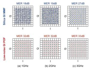
Figure 2. Constellation map for signal transmitted through 100-m silica GI MMF and 100-m low-noise GI POF. Carrier frequencies are (a) 1 GHz, (b) 2 GHz, and (c) 3 GHz.
