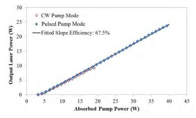
Figure 3: Slope efficiency of Ho:YAG SC fiber[9]
