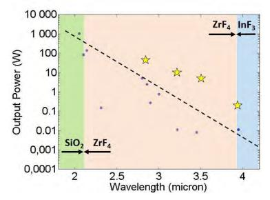
Figure 1. Maximum cw output power from mid-IR fiber lasers as a function of wavelength.
