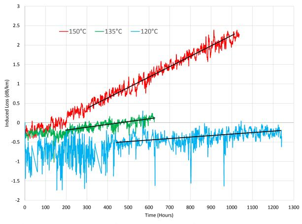
Figure 3. Induced loss @ 1244nm of 3 carbon-coated VHM2000 fibers, exposed to 84.7atm pure  $H_2$  at different temperatures
