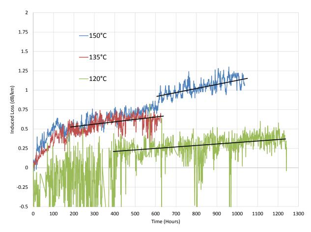
Figure 5. Induced loss @ 1064nm of 3 carbon-coated VHM2000 fibers, exposed to 84.7atm pure  $H_2$  at different temperatures
