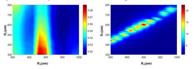
Figure 2 Loss of fundamental mode (a) and HOM (b) changing with Ra and Dc
