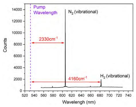
Figure 3. Results of a Raman measurements made with fiber A showing the nitrogen and hydrogen vibrational Raman emission (1<sup>st</sup> Stokes) lines at ~2330cm<sup>-1</sup> (N<sub>2</sub>) and 4160cm<sup>-1</sup> (H<sub>2</sub>).
