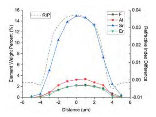
Figure 2. Composition profiles measured by WDX and fiber RIP with 0 µm corresponding to the fiber core center.
