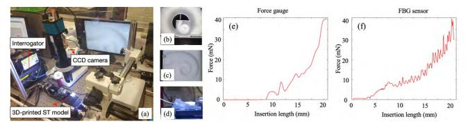
Figure 2. (a) Experimental setup used for the in-vitro tests, (b) a 3D scala tympani (ST) phantom printed by a 3D printer, (c) 2D ST phantom, and (d) 3D ST phantom considering otologic positioning during surgery. (e) and (f) plot the measured tip contact force using external force gauge and internal FBG sensor as a function of insertion length, respectively.
