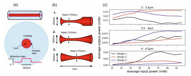
Figure 1. (a) Cross section of silicon fiber showing core, cladding and interface layers. (b) 1-3 show the three taper designs (core dimensions only). (c) Power outputs of simulations in three wavelength ranges according to input power. Black lines show Design 1, red lines Design 2 and blue lines Design 3.
