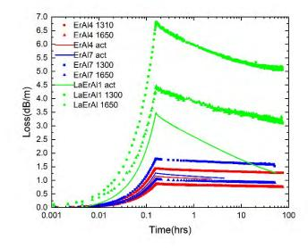
Figure 3. Growth and recovery of the loss of output optical power (active) and radiation-induced absorption measured spectrally at 1.31 and 1.65 µm.
