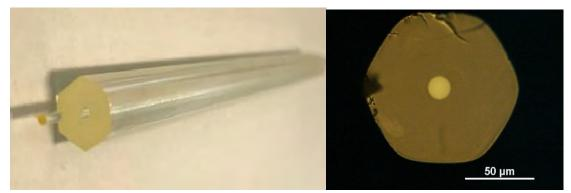
Figure 2.a) Cross sectional view of the extruded hexagonal inner cladding with the core rode inside. b). Optical microscope image of the fabricated Tm doped Germanate LMA single mode fiber.
