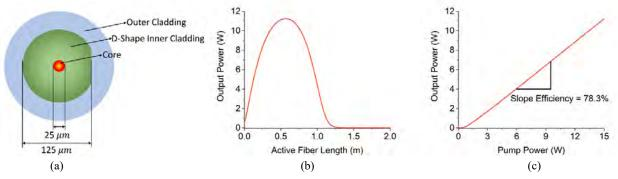
Fig. 5. (a) Cross section of the fluorosilicate double-clad fiber (b) output power versus active fiber length with 15W of pump power (c) output power versus pump power with 0.78m fluorosilicate double-clad fiber.
