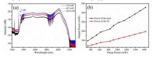
Fig.3 (a) Spectra of the SC from the HNLF with different pump power of the 1480 nm Raman Laser. (b) Output power of the NLP mode locked fiber laser and power of the SC from the highly nonlinear fiber.
