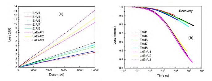
Figure 1. Example data of the (a) growth and (b) recovery of the loss of 1.48 µm pumped MOPA output optical power for various EDFs. Because of the differences in peak losses, the recovery has been normalized to the peak value.
