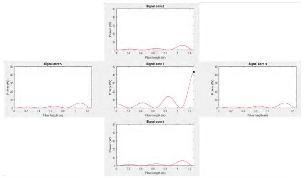
Fig.2. Simulation of the power evolution along the different cores of the proposed Talbot fiber.
