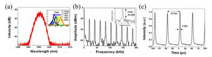
Figure 2. Q-switching fiber laser output at 458.5mW power pump. (a) Optical spectrum analyzer data (b) RF spectrum data (c) oscilloscope trace data
