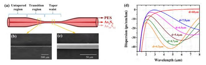
Figure 1. (a) Schematic of a ChG tapered fiber with a decaying-exponential profile. (b) SEM image of a part of transition region for a tapered fiber. (c) SEM image of the taper waist for a tapered fiber. (d) Calculated fundamental mode dispersion characteristic curves of ChG fibers with various core diameters.
