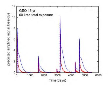
Figure 5. The predicted signal loss (red) in an EDFA made with LaErAl1 on-orbit in GEO exposed to a number of solar flares over a 15-year lifetime together with 95% confidence bounds (blue).
