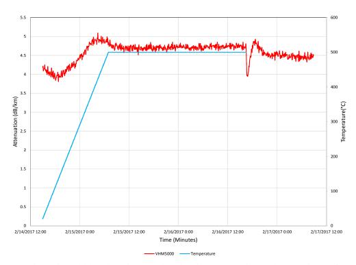
Figure 4: VHM5000 with gold-based coating, 43m length, 850nm attenuation, 34 hours at 500°C after soaking at 500°C for 900 hours
