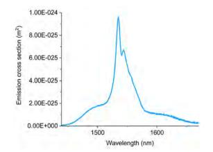
Figure 4. Emission cross section spectrum measured for Fiber 1. The emission spectrum is relatively narrow compared with aluminosilicate glasses [14].
