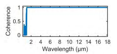
Figure 3. Simulated first-order coherence with the pump wavelength of 10  $\mu$ m and coupled pump peak power of 1.3 MW.
