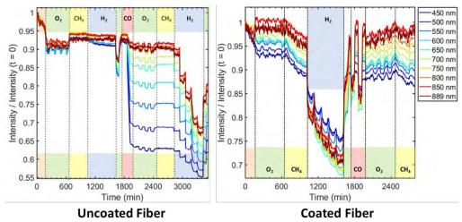
Figure 7: Normalized transmission spectrum for spinel-coated and uncoated fiber for gas exposure test[15].
