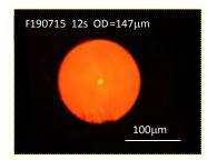
Figure 7 The near field photo of a fiber sample.
