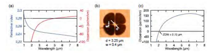
Figure 4. (a) Refractive index and material dispersion spectra of  $As_2S_5$  glass. (b) Cross-section photograph of the Ch-SCF. (c) Chromatic dispersion spectrum of the fundamental mode in the Ch-SCF. The ZDW was located at 2.12  $\mu$ m.
