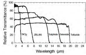
Figure 1. Infrared transmission for several bulk glass samples, thickness of about 2-3 mm [2]
