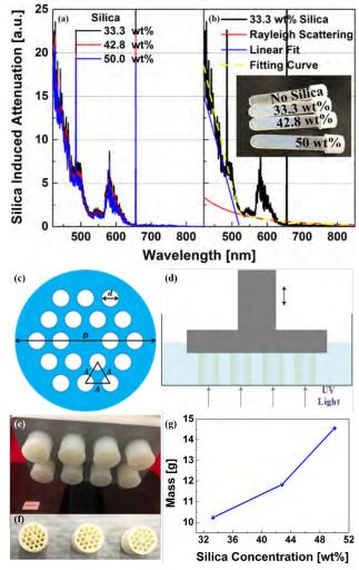
Fig. 1. (a) Silica induced attenuation of resins using plastic cuvettes; (b) Rayleigh and linear fitting of attenuation, insert: resins photo; (c) Designed preform structure; (d) DLP 3D printing; (e) preforms after 3D printing. (f) Preforms after cleaning; and (g) the preform mass vs silica concentration.
