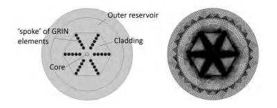
Figure 1. Example of the fiber design geometry (left) and the corresponding mesh (right) in COMSOL. The high index GRIN elements extend out from the core in the center of the design and are surrounded by the background region. The ends of the GRIN element 'spokes' are located close to a raised index region that serves as a reservoir for the outcoupled light.
