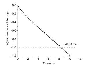
Figure 3. Fluorescent lifetime in the erbium-doped fluorosilicate fiber.
