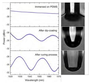
**Figure 1.** Back-reflected spectra obtained during the end-cap deposition on the tips of single-mode fibers. Note that the spectra include results obtained from three different probes fabricated using the same immersion parameters. The images show the fiber tip during immersion, after extraction from the PDMS and after curing.
