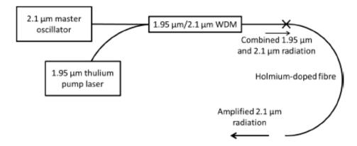
Figure 1: Forward pumped, core-pumped configuration where the master oscillator and the thulium pump laser are coupled into the fundamental mode of the core of a holmium-doped fibre via a fused biconic taper.
