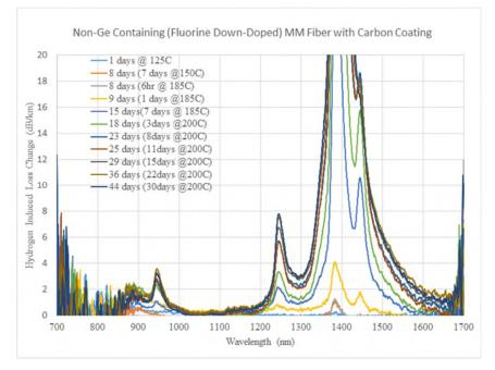
Figure 5: Hydrogen induced loss in a non-GE containing "Pure-core" MM graded index fiber
