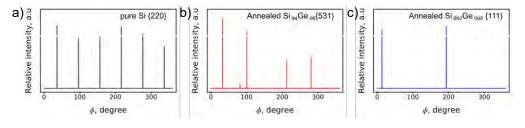
Fig. 2 XRD results on fibers a) pure silicon single crystal core fiber, b) annealed Si<sub>.94</sub>Ge<sub>.06</sub> with small secondary crystal and c) single crystal annealed Si<sub>.992</sub>Ge<sub>.008</sub>. The {hkl} indicate the Bragg peak for each phi scan.
