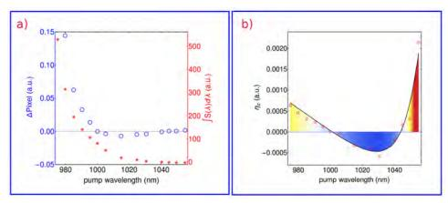
Figure 2. a) Blue circles are the  $\Delta Pixel$  of the thermal camera at each wavelengths, and red asterisks are the integrate under the  $S(\lambda)$ . b) Measured and fitting of the cooling efficiency ( $\eta_c$ ) for the Yb:ZBLAN fiber. The solid curve shows a fit of  $\eta_c$  and the red circles shows data points at different wavelength.
