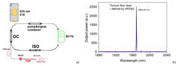
Figure 1. a) Schematic diagram of the experimental setup, and b) output of Tm fibre laser.
