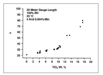
Figure 4. Fatigue resistance as a function of TiO<sub>2</sub> in the cladding.
