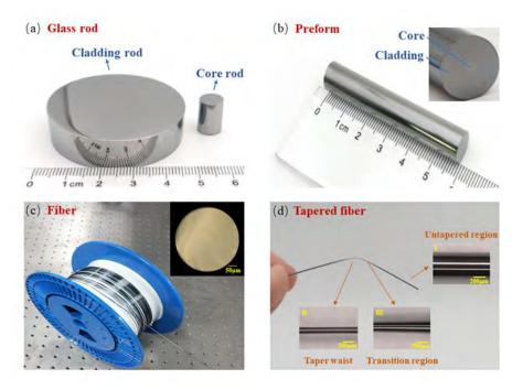
Figure 2. (a) Core and cladding glass rods. (b) Extruded preform. Inset: cross-section of the preform. (c) A roll of well-fabricated step-index fiber. Inset: cross-section image of the fiber. (d) Tapered fiber with the core waist diameter of 80µm. Inset: I untapered region, II taper waist, III transition region.
