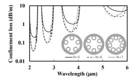
Figure 1. Calculated confinement loss spectra of the fundamental mode with different value of N (5, 6 and 7).
