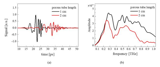
Figure 3. (a) Measured time-domain waveform of THz pulse passing through the porous tube. (b) Corresponding amplitude spectrum.
