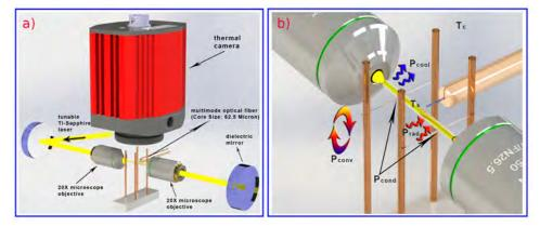
Figure 1. a) Experimental setup for LITMoS test of the Ytterbium doped ZBLAN fiber. b) Magnified fiber holder part and illustration of three source of heat load, convective, conductive and radiative
