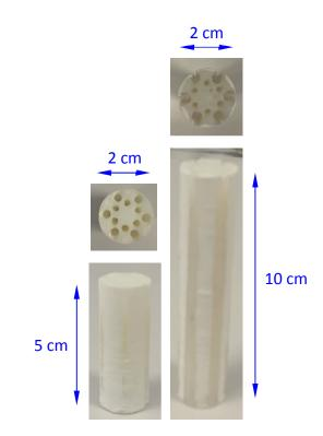
Figure 2. Raw silica fiber preforms fabricated using the UV curable resin with a DLP 3D printer.
