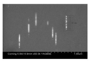
Figure 10; SEM image of the resulting elongated particles
