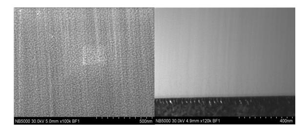
Figure 1. Tunneling electron microscope image of a typical spinodally phase-separated aluminosilicate fiber core (left) and pure silica cladding (right). The nano-scale phase separation in the core is evident from the image.
