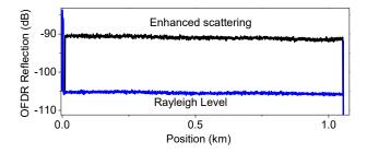
Figure 2. OFDR trace showing more than 10 dB increase in reflected power over 1.1 km of UV processed fiber (black curve). The blue curve shows the level of the native Rayleigh scattering in the bare fiber.
