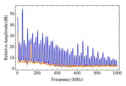
Figure 6. RF beat spectra taken at a laser output power of 2 mW for the laser without (blue) and with (orange) the P-SF. The beat signal between the large number of cavity modes, spaced at the laser free spectral range (~ 16 MHz) are clearly visible. These modes are suppressed in the case of the random laser. At the highest power the spectrum exhibits a random presence of one or two peaks, at random frequency. Such is an example that is shown here.
