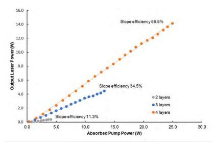
Figure 4: Slope efficiency of Ho:YAG fibers grown from a preform with different number of HoAG layers[10]
