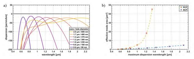
Figure 2: A) Dispersion curves for various combinations of core and hole diameters for four suspending struts with a thickness of 1/6<sup>th</sup> of the core diameter. B) Effective mode area as a function of dispersion high point location also known as maximum dispersion wavelengths.
