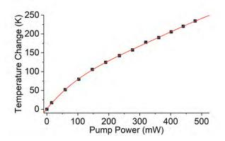
Fig. 1. Temperature change of 2.4mm HF with different pump power, the dots are measured data and the line is a polynomial fit to the data meant as a visual aid to the reader.
