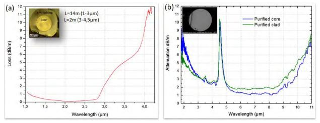
Figure 1. Attenuation curves of: (a) the large core (TZNF) step-index tellurite fiber; (b) both single index chalcogenide fibers from core GST20 and clad GST10 glasses.
