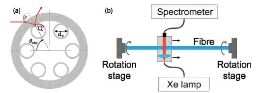
Figure 1: (a) Path of a ray refracting at point P, which at point Q excites a WGM inside a capillary. The ray exits the fiber at a specific angle, allowing detection of the WGM spectrum of the selected capillary. (b) Setup used to scan along a fiber length while rotating the fiber to selectively measure individual capillaries.
