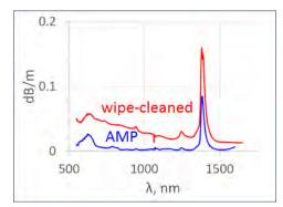
Figure 3 Losses of fibers drawn from wipe-cleaned and AMP-cleaned preforms. From [5].
