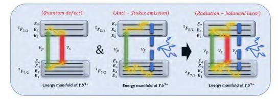
Figure 1. Schematic of radiation-balancing process in a laser with a Yb-doped gain. As it is obvious, quantum defect which is an intrinsic process in a laser can be canceled out simultaneously by anti-Stokes fluorescence cooling.
