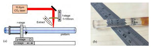
Figure 1 (a) Showing a conceptual schematic of the  $CO_2$  preform processing system. The preform itself is mounted within a rotation stage mounted onto x-y translation stages. The QCW pulsed  $CO_2$  laser is directed via a focusing lens onto the top surface of the preform. (b) An example of a 12mm diameter preform shaped to an octagonal outer profile.
