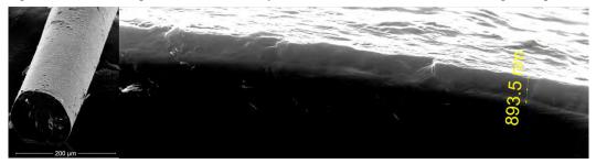
Figure 6: Spinel coated sapphire fiber. Magnified image showing the spinel film on fiber.
