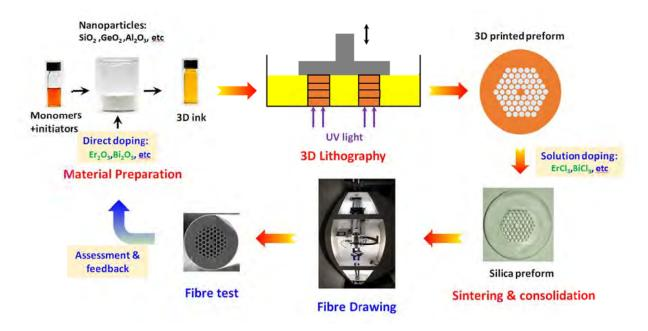
Figure 1. 3D lithography-based new pathway to silica optical fiber fabrication.
