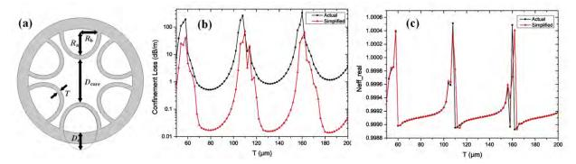
Figure 1. (a)Schematic diagram of ARF with six half-ellipse cladding tubes. (b, c) CL and Neff\_real changing with the shell thickness of cladding tubes.
