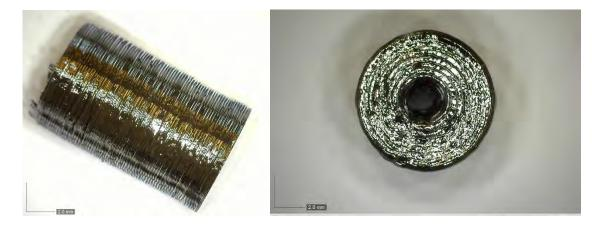
Fig 1. Photos of the chalcogenide glass hollow preform obtained by 3D printing.
