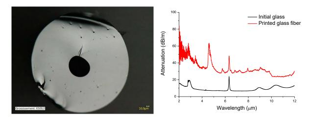
Fig 2 : 3D-printed chalcogenide hollow fiber : (a) fiber cross section, (b) : Optical loss of the chalcogenide (black) and the printed hollow fiber (red).
