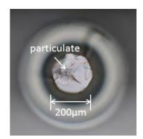
Figure 1 Cross section of fiber that failed at roughly 300W, showing an embedded particulate that likely have generated the failure.
