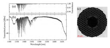
Fig. 1: (a) Transmittance of water vapour from HITRAN database (1 ppm, 1 km, 0.05 nm filter) (b) transmitted spectra recorded at 0.05 nm resolution and (c) scanning electron micrograph of PBGF-A (55 m).
