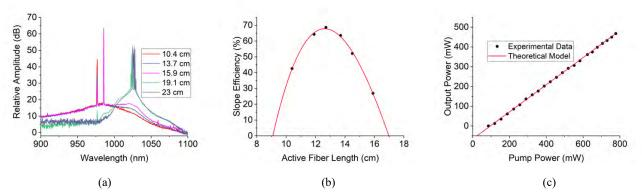
Fig. 4. (a) Output spectra with different active fiber lengths. (b) slope efficiency with different fiber lengths (the curve is a polynomial fit and only for visual aid). (c) Experimental and theoretical output power versus launched pump power at the near-optimized active fiber length.
