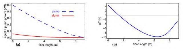
Figure 4. (a) Propagation of right and left moving pump and signal powers along the single-pass pump C/C Yb-doped ZBLAN fiber amplifier at  $\lambda_p = 1020$  nm and  $\lambda_s = 1050$  nm with  $P_{p0}^+ = 0.5$  kW, (b) Longitudinal temperature distribution ( $\Delta T$ ) of the single-pass pump C/C Yb-doped ZBLAN fiber amplifier.
