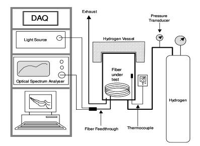
Figure 1. Real-Time Hydrogen Ingression Test Setup
