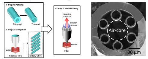
Figure 4. Schematic diagram for the fiber fabrication of tellurite HCOF with a 6 non-touching cladding air-hole structure and the cross-sectional image of the fabricated tellurite HCOF taken by a scanning electron microscope.
