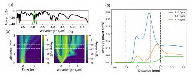
Figure 2. (a) Output SC (green line is input spectrum, red dashed line shows -30dB level), (b) temporal evolution and (c) spectral evolution with 17.3mW (5.75kW peak) 130fs pulses in Design 1. (d) Power evolution of the mid-IR ranges of interest. Dashed lines show the ends of the down-taper, waist and up-taper.
