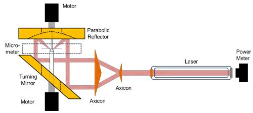
Figure 1: Schematic of Laser Heated Pedestal Growth Set-up
