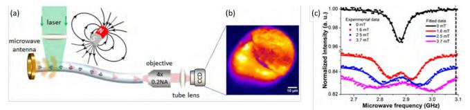
Figure 5. Optically detected magnetic resonance (ODMR) of ND doped tellurite fiber. (a) Schematic of experimental set-up for ODMR measurement using laser light at 532 nm for side excitation and (b) imaging the NV emission from the endface onto an camera. (c) ODMR spectra from a ~200  $\mu$ m<sup>2</sup> region of the fiber for varying external magnetic fields. The square points are measured data, and the solid lines are fitted curves. Figure after [29].
