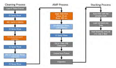
Figure 2 Flow diagram for AMP process. From [5].
