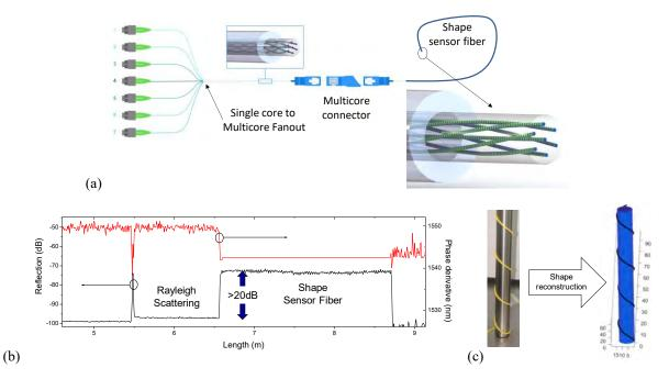
Figure 1. (a) Shape sensing components: Single- to multi-core fanout, multi-core connectors, and shape sensor fiber. (b) OFDR trace showing increased scattering (black trace) and improved signal-to-noise ratio of the spatial phase derivative signal (red curve) in the shape sensor fiber. (c) Shape reconstruction: Fiber wound around a post (left); reconstructed shape (right).
