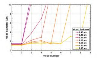
Figure 3: Modal diameter simulation for the first nine modes (including polarization discrimination) for various strut thicknesses. The fiber has a core diameter of 2µm. Modes with significant larger diameter are not located in and hence guided by the core.
