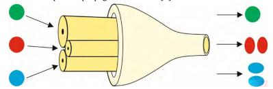
Figure 1. Schematic mode-selective photonic lantern made by fusing and tapering three dissimilar SMFs in an F-doped capillary.
