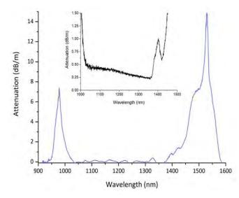
Figure 2: Attenuation plot of the metal-derived EDF over the region of 900 - 1700 nm. Inset is a magnification of the region of lowest loss between 1000 - 1500 nm.
