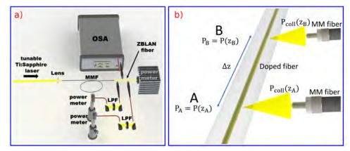
Figure 3. a) Schematic of the experimental setup which is used for the MACSLA method. OSA stands for optical spectrum analyzer, LPF for long-pass filter, and MMF for multimode fiber. b) Schematic of the propagation of the pump power in the core of the optical fiber. And collecting the spontaneous emission from the side of the Yb-doped ZBLAN fiber by two multimode passive optical fibers.
