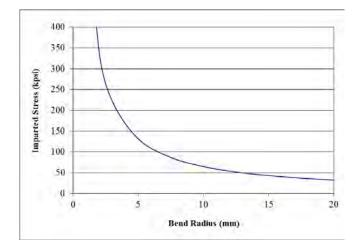
Figure 2. Imparted Stress as a function of bend radius for a 125 µm diameter fiber.
