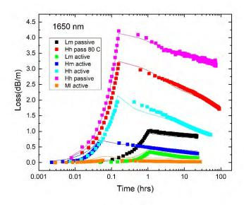
Figure 4. Results of 7 experiments with the LaErAll NP-doped fiber using different dose rates (L, M, H = 0.5, 2.5, 500 Gy/h) and total doses (l, m, h = 10, 30, 100 Gy) together with the fits obtained via the statistical kinetics model. The lines are the data and the points are the fit.
