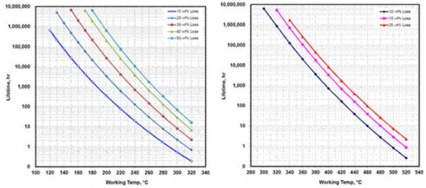
Figure 1. TGA for MTA (LEFT) and polyimide coating (RIGHT) used on BHGE CoreBright fibers.
