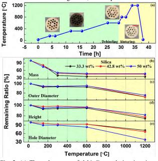
Fig. 2. (a) Thermal process of debinding and sintering, inset photos: preforms of 33.3 wt% silica after thermal treatment at 150, 300, 600 and 1200 °C. (b) ~ (e) Remaining ratio of mass, outer diameter, height and hole diameter after thermal treatment in (a).
