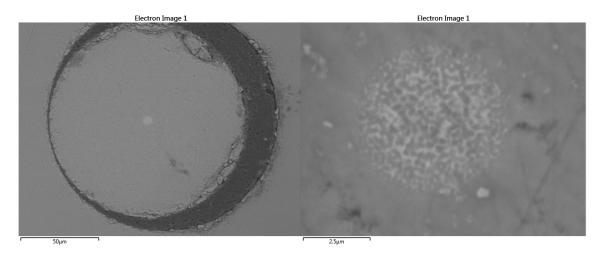
Figure 2. Scanning electron microscope image of the calcium silicate fiber core (roughly 5 µm diameter). Note the larger scale relative to the aluminosilicate fiber. The sizes of the particles were on the order of 250 nm.
