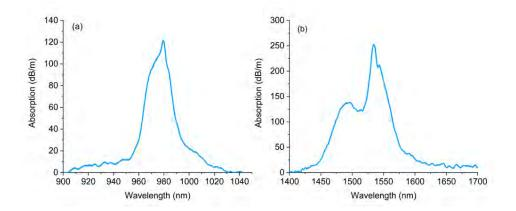
Figure 5. Fiber 1 absorption spectrum in infrared region (a) 900-1050 nm and (b) 1400-1700 nm.
