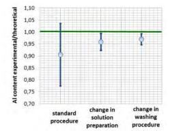
Figure 1: Impact of changing preparation of solution and subsequent washing procedure of doped particles on reproducibility of Al<sub>2</sub>O<sub>3</sub>-doped SiO<sub>2</sub> powder. The given Al-content is the average *EPMA* value measured in a line scan over the preform core diameter.
