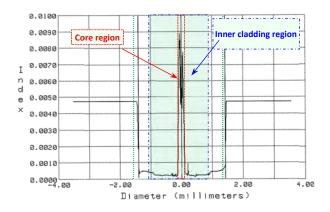
Figure 6. Index profile of the fiber tip at the start of fiber draw.
