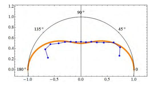
Figure 3. Normalized scattering pattern measured at 532 nm for the aluminosilicate optical fiber (blue) shown with the normalized Rayleigh pattern from theory.
