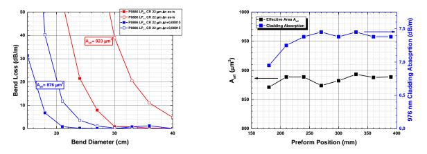
Fig. 2.a: LP01 & LP11 bend loss as a function of bend diameter Fig. 2.b: Aeff and cladding absorption evolutions along the preform length
