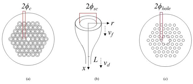
Figure 1 Illustration of (a) an SOF structure with the inner capillary diameter  $2\phi_c$ ; (b) a single capillary with inner diameter,  $2\phi_{sc}$  at the neck-down region; (c) a fabricated hexagonal structured optical fibre, SOF with inner diameter  $2\phi_{hole}$ .
