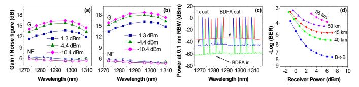
Figure 1. (a,b) BDFA gain and noise figure for 500 and 800 mW pump power; (c) 40 km transmission spectra, note wavelength shift was added to increase visibility; (d) BER vs power for 40-55 km distances.
