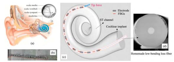
Figure 1. (a) Schematic figure of a cochlea with an implant system<sup>1</sup>: 1) a speech processor, 2) internal receiver, 3) the electrode array, 4) the auditory nerve. (b) The microscopic photo of an actual cochlear implant used for surgery. (c) The schematic figure of the cochlear implant integrated with fibre Bragg grating (FBG) sensors. (d) SEM photo of the fabricated fibre.
