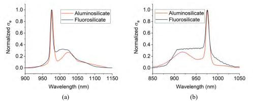
Fig. 1. Normalized (a) emission cross section ( $\sigma_e$ ) and (b) absorption cross section ( $\sigma_a$ ) spectra for Yb-doped commercial aluminosilicate fiber and the fluorosilicate fiber (studied in this work)
