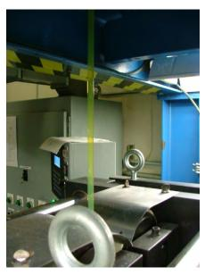
Figure 3; a glass redraw apparatus
