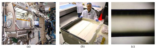
Figure 1. (a) Fiber manufacturing payload by FOMS Inc. inside Microgravity Science Glovebox on board of ISS, (b) unpacking of two manufacturing units in Houston, TX after returning back to Earth, (c) fluoride optical fiber produced in microgravity.
