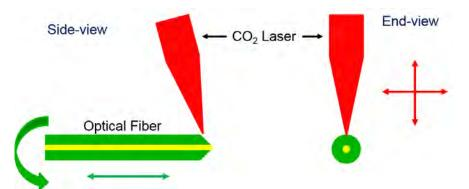
Figure 1. The schematic of wedge-shaped fiber lenses based on CO<sub>2</sub> laser glass ablation. The green arrows show the rotating and moving directions of the optical fiber; and the red arrows represent the moving directions of the CO<sub>2</sub> laser beam.
