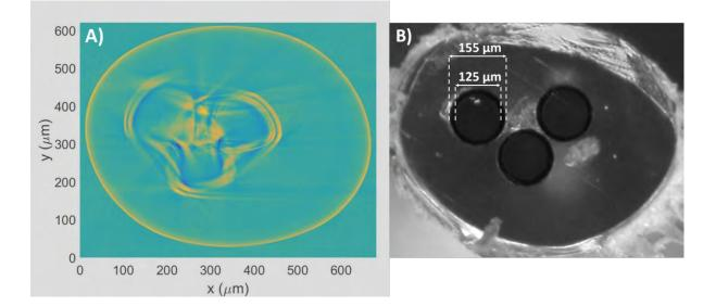
Figure 3: A) Sliced view of the coated triplet obtained applying an inverse Radon transform on the tomogram shown in Fig.2. B) Direct image of the coated triplet polished face.
