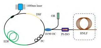
Fig. 1. Configuration of the all-fiber NLP mode locked fiber laser based on nonlinear amplifying loop mirror. EDF: Erbiumdoped fiber; OC: optical coupler; PC: polarization controller; OR: optical reflector; ISO: isolator; WDM: wavelength division multiplexer; HNLF: highly nonlinear fiber.
