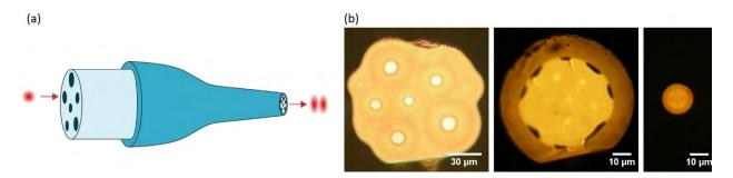
Figure 2. (a) Schematic mode-selective photonic lantern made by tapering a multicore fibre with dissimilar cores in a fluorine-doped jacket. (b) Cross-sectional micrographs of (left) the 6-core fibre, (centre) a point partway down the photonic lantern's taper transition and (right) the lantern's multimode output.
