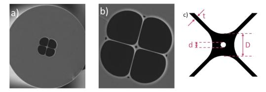
Figure 1: Scanning electron microscopy images of a) the full suspended-core fiber and b) the central section containing air holes. Design parameters are depicted in c).
