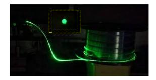
Figure 8 The light transmission of the optical fiber when launched with 532nm. The inset is the far field pattern of the fiber.
