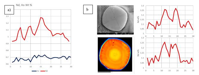
Figure 5a: Radial auto-segregation of ions in Nd, Ho:YAG; Figure 5b: Cross-section and radial auto-segregation in Nd:YAG
