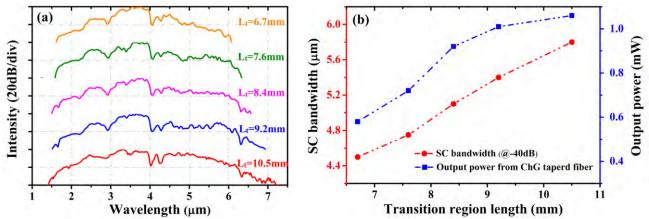
Figure 4. (a) Measured SC spectra generated from 12-cm-long As-S ChG tapered fibers with transition region length varying from 6.7 mm to 10.5 mm pumped at  $3.25 \ \mu m$ . (b) Bandwidth of the generated SC spectra at -40dB and the corresponding output power from tapered fibers as a function of transition region length.
