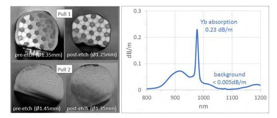
Figure 4a Mixtures of Yb doped glass (brighter regions) and F-doped glass (darker region). After mixing twice (Pull 2), a cane was built into a cladding-pumped optical fiber. Figure 4b suggests that the losses of the cladding-pumped fiber are suitably low for high power applications.
