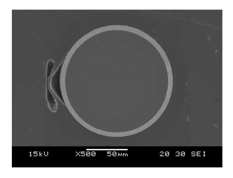
Figure 1: SEM cross-section of fiber produced using the current process
