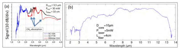
Figure 2. (a) SC generated in the step-index tellurite fiber measured with an OSA (blue line) and a FTIR (dark line). Red line shows the SC travelling into the  $CH_4$ -filled gas cell. (b) SC generated in the chalcogenide step-index fiber.
