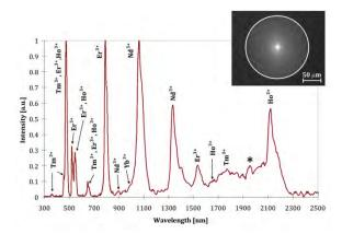
Figure 1. Typical fluorescence spectrum of a single-core, multi-dopant fiber containing Nd<sup>3+</sup>, Ho<sup>3+</sup>, Tm<sup>3+</sup>, Er<sup>3+</sup>, and Yb<sup>3+</sup> pumped at 800 nm.
