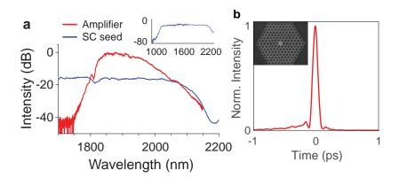
Figure 1. (a) Logarithmic spectrum of the long-wavelength part of the low noise SC seed pulse generated in all-solid, allnormal dispersion photonic crystal fiber and spectrum after subsequent amplification in an all-fiber chirped pulse amplifier. The complete SC spectrum is shown in the inset, supporting a single-cycle (5 fs) pulse. (b). Reconstructed pulse with 66 fs duration at the exit of the amplifier. The inset shows a microscope image of the PCF used for SC generation.
