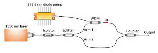
Fig. 2. Experimental Setup
