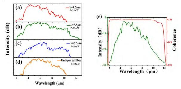
Figure 5. Measured SC spectral generated from Te-based ChG tapered fiber with different pumping wavelengths of (a) 4.5  $\mu$ m, (b) 5.5  $\mu$ m, and (c) 6.5  $\mu$ m and (d) an untapered fiber pumped at 5.5  $\mu$ m.(e) Simulated the SC spectrum (green curve, left axis) and its coherence property (red curve, right axis).
