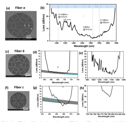
Fig.1. Ultralow loss CTFs. (a, c, f) Scanning electron microscope (SEM) image of fiber *a*, *b* and *c* respectively. (b, d, e, g, h) Measured loss spectra. The gray stripes in (d) and (g) outline the RSL range of SGF. The star symbols represents the loss level of commercial SGF.
