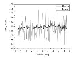
Figure 2: Dopant profiles of Al<sub>2</sub>O<sub>3</sub> by EPMA for the REPUSIL process and the novel plasma based approach.
