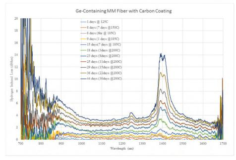
Figure 4: Hydrogen induced loss in a typical GE containing MM graded index fiber
