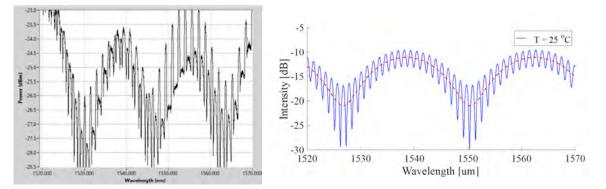
**Figure 4.** Measured reflected spectra from the microbubble PDMS end-capped fiber sensor (left). The spectrum obtained using a three-mirror F-P device (right) shows similar features to those obtained with the fabricated sensor.
