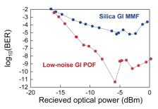
Figure 3. BER as functions of received optical power for MMF links with silica GI MMF and low-noise GI POF.
