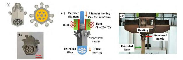
Figure 1. (a) Structured nozzle design including a 3D model and a bottom-view, from left to right respectively. Yellow colors represent the cross-section of the extruded fiber from structured nozzle. (b) Metal 3D printed structured nozzle. (c) Schematic and (d) photograph of the experimental setup used to extrude HC-MPOF.
