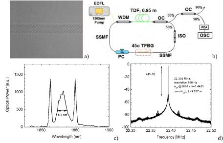
Figure. 2. a) Microscope picture of the TFBG inscribed using the pl-by-pl inscription method, b) schematic diagram of mode locked fibre laser system. c) Optical spectrum of the laser output and d) RF spectrum at 100 Hz resolution.
