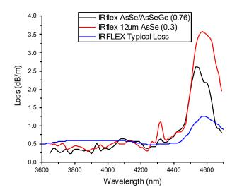
Figure 2. Loss spectra for three As<sub>2</sub>S<sub>3</sub> chalcogenide fibers.
