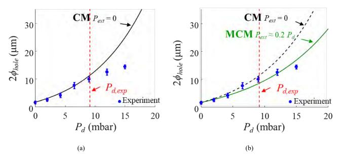
Figure 2. Experimental vs predicted results of the single capillary model at  $T_d = 1860$  °C,  $P_d = (0.1-16)$  mbar: (a) Ignoring  $P_{ext}$  and (b) with  $P_{ext} \approx 0.2P_d$ .
