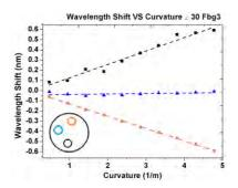
Fig. 3a. Core 3 lies on the neutral axis, core 1 experiences strain, and core 2 compression
