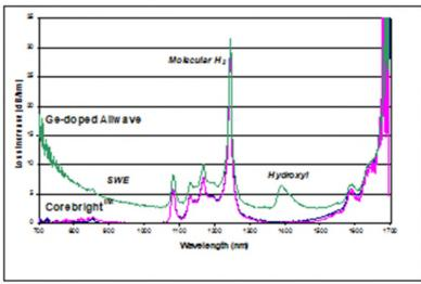
Figure 2: Hydrogen induced loss in Germanium containing SMF and in pure core Corebright SMF.
