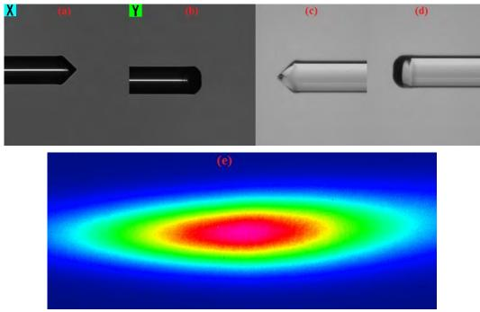
Figure 2. (a) & (b) The images of the wedge-shaped fiber lens in the splicer; (c) & (d) the images in the microscope; (e) the beam profile taken with a Gentec camera.
