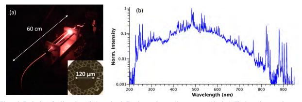
Figure 3: Excitation of a 60 cm long discharge in a helium/neon mixture at low pressure (10 mbar). The inset shows a microscope image of the HC-PCF cross section. (b) Spectrum of an atmospheric pressure discharge of a helium / xenon mixture, recorded at the fiber exit open to the atmosphere.
