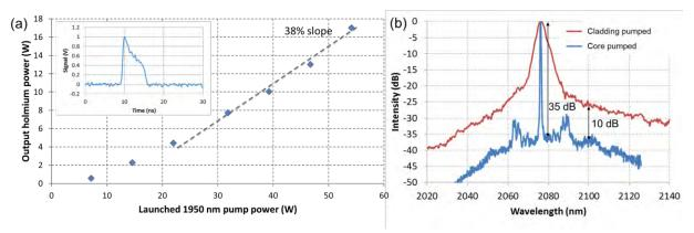
Figure 3: (a) Output power vs launched pump power from a pulsed holmium amplifier; Inset: Output pulse showing a 5 ns duration and exhibiting significant gain shaping. (b) Output spectrum at 36 kW peak power showing the reduction of spectral broadening comparing a previous cladding-pumped amplifier with a core-pumped amplifier approach.
