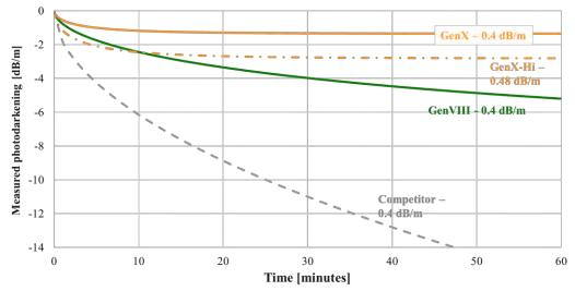
Figure 3. Accelerated PD measured in various 20 µm core YDF with nominal cladding absorption of 0.4 dB/m at 915 nm GenVIII and GenX correspond to two different Yb-doped glass compositions. GenX+ has 20% higher cladding absorption that GenX.
