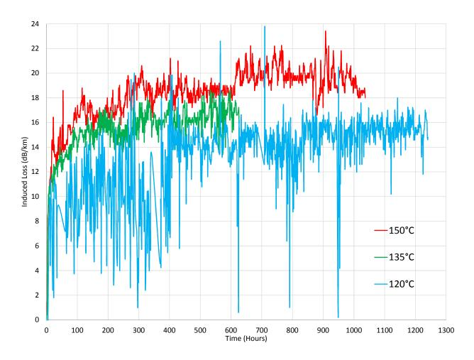
Figure 4. Induced loss @ 1064nm of 3 non carbon-coated VHM2000 fibers, exposed to 84.7atm pure  $H_2$  at different temperatures
