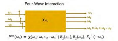
Figure 6: schematic of a nonlinear induced four wave mixing
