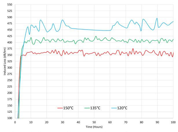
Figure 2. Induced loss @ 1244nm of three non carbon-coated VHM2000 fibers, exposed to 84.7atm pure  $H_2$  at different temperatures
