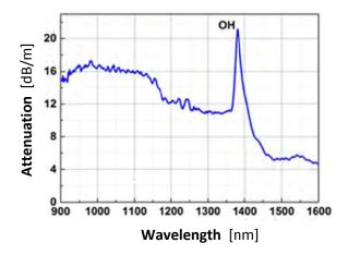
Figure 9. Measured spectral attenuation of one of the 1<sup>st</sup> step-index fiber draw from 3D printed silica preforms.
