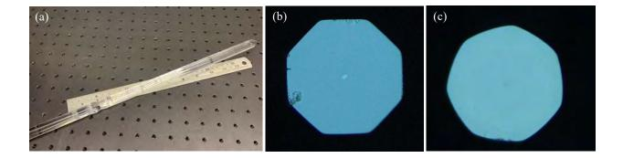
Figure 2. (a) Image of a 300mm long preform shaped into three sections with varying outer cladding geometries. (b) End face image of a fiber drawn from a  $CO_2$  laser shaped preform, (c) End face image of a fiber drawn from a 7 sided Reuleaux polygon  $CO_2$  laser shaped preform.
