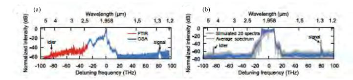
Figure 5. (a) Experimental observation of the wavelength conversion when the pump wavelength is at 1.958 µm in the normal dispersion regime. Red and blue curve indicate measured spectrum with FTIR and OSA, respectively. (a) Numerical observation of the wavelength conversion in the Ch-SCF. Blue curve indicates an average spectrum. Individual realizations employed in the average spectrum are shown in gray curves.
