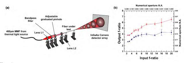
Figure 4. (a) Schematic of the FRD measurement experimental setup. (b) Output f-ratio versus input f-ratio measured for the 6-mode step-index fibre (blue squares) and the 6-mode MSPL device (red points). Points are an average of five measurements with the maximum and minimum values measured represented by the error bars.
