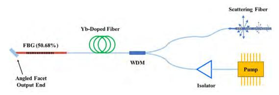
Figure 4. Random laser configuration. The commercial Yb-doped fiber is end pumped by a laser diode at 976 nm. The broadband isolator was used to prevent lasing from the pump diode facet. The output was taken at the FBG end.
