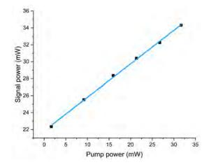
Figure 6. EDFA output power versus pump power with saturated signal input power. The slope efficiency is about 39.6%. A major source of loss is believed to originate from poor mode matching between the active EDF and the EDFA system fiber.
