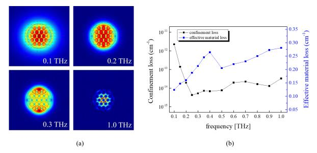
Figure 2. Mode distribution of the porous tube with PTFE depending on the frequency. In the low frequency band, the mode is distributed evenly in the air holes of the tube.
