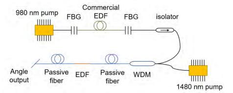
Figure 1. EDFA system setup for measuring the slope efficiency of EDF.
