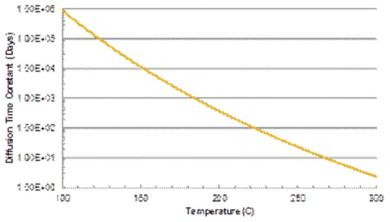
Figure 3: Typical diffusion time through high quality carbon coating vs temperature.
