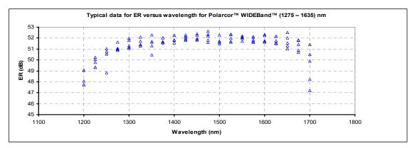
Figure 11; extinction ratio in db vs. wavelength
