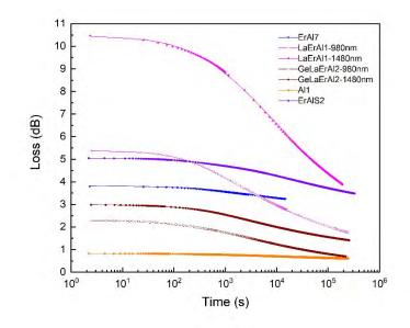
Figure 2. Recovery of the radiation-induced loss (points) and fits to n<sup>th</sup>-order kinetics (lines).
