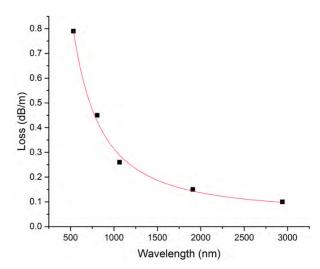
Figure 2: Total attenuation losses for a 1 meter long 330 µm diameter YAG SC fiber at different wavelengths
