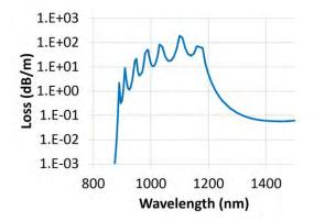
Figure 2. Calculated losses from COMSOL modeling showing loss exceeding 1 dB/m between 0.9 µm and 1.2 µm.
