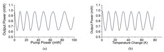
Fig. 3. (a) Output power versus launched pump power to HF. (b) Output power versus temperature change of HF
