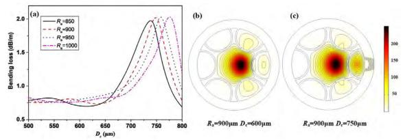
Figure 3 (a) Bending loss of ARF changing with cladding tubes when the bending radius is 50cm. The electric field distribution of fiber cross section when  $R_a$  is 900 µm, Dc is 600 µm(b) and when  $R_a$  is 900 µm, Dc is 750 µm(c).
