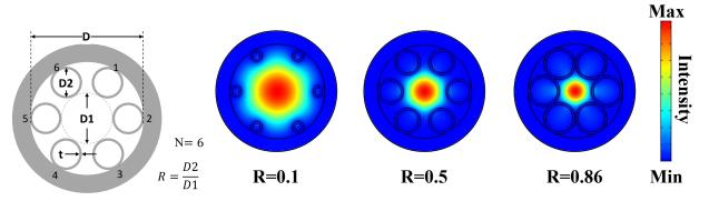
Figure 2. Calculated intensity distribution of the fundamental mode in the air-core when N=6 and R=0.1, 0.5 and 0.86, respectively.
