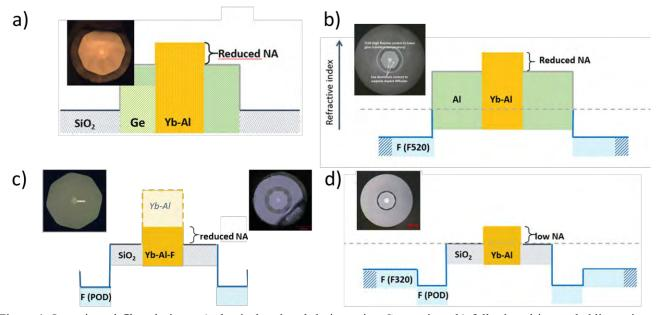
Figure 1. Investigated fiber designs: a) classical pedestal design using Germanium, b) fully doped inner cladding using Al-doped REPUSIL material, c) Fluorine-codoped core for refractive index reduction, d) low Yb<sub>2</sub>O<sub>3</sub> concentration (0.08 % molar).
