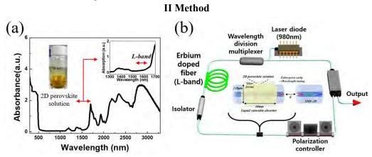
Figure 1. (a) 2D perovskite 40wt% solution VIS-NIR spectrum (b) the fabrication process of 2D perovskite liquid saturable absorber and configuration of a laser ring cavity
