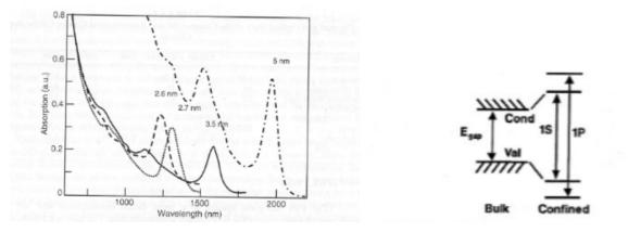
Figure 7; position of the energy level splitting as a function of the dot size<sup>32</sup>
