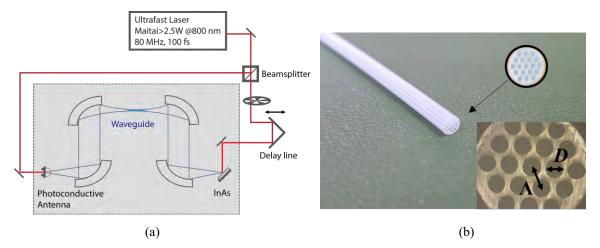
Figure 1. (a) A diagram of the optical set-up for waveguide measurements. (b) Photograph showing the porous PTFE tube constructed. Upper right-hand corner inset shows the cross-section of the tube where 17 air holes are arranged. Lower right-hand is the enlarged cross-section.
