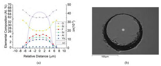
Fig. 2. (a) Compositional and refractive index profiles and (b) SEM micrograph of the Yb-doped fluorosilicate fiber.
