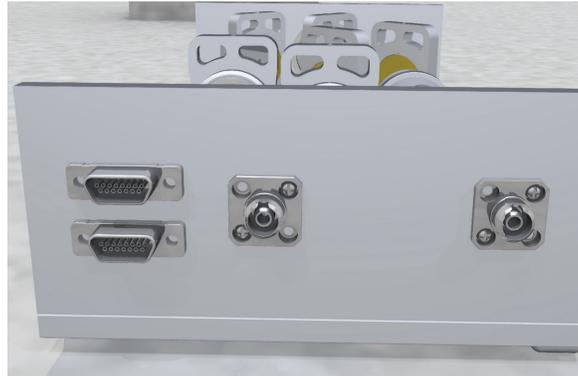
Figure 9: Electrical and optical interfaces on the optical system cover
