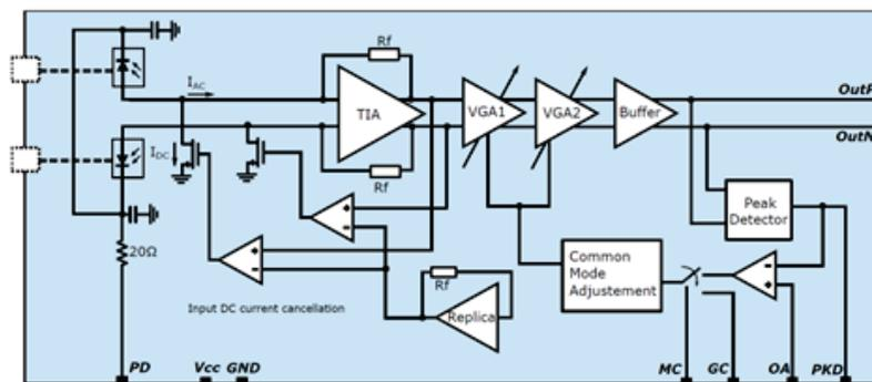
Figure 8: Block diagram of the Rx-ePIC electronics block
