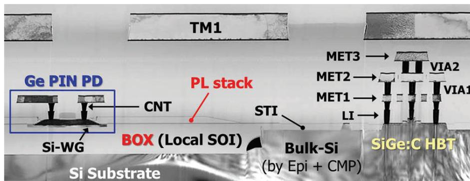
Figure 5: Cross-section of an EPIC's mixed substrate
