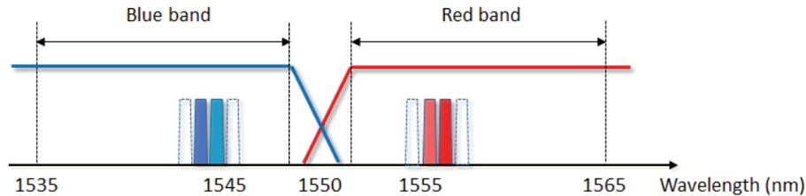
Figure 1: Typical OISL wavelength allocation for bi-directionality
