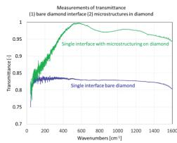
Figure 2. (Left) Uncoated diamond sample, (Right)Transmittance of single interface bare diamond compared to bare diamond including microstructuring versus wavenumber – Concept A
