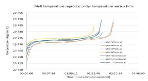
Figure 8 (Left) Phase change cell mock-up for plateau repeatability measurement, (Right) Melt temperature reproducibility within 10 mK measurement results - Concept A
