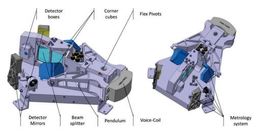
Figure 12. FORUM FSI interferometer sketch – Concept B. (Courtesy OHB)
