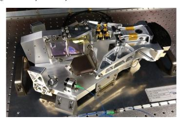
Figure 14. FORUM Interferometer mechanism breadboard Concept B. (Courtesy of OHB).
