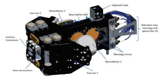
Figure 11. FORUM FSI Interferometer breadboard sketch - Concept A. (Courtesy ABB).
