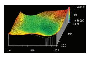
Figure 4 (Left) FSI diamond beamsplitter Efficiency based on measurement (Concept A), (Right) Ge-coated diamond WFE measurement in reflection on full scale sample) – WFE measured <100 nm rms (Concept B)
