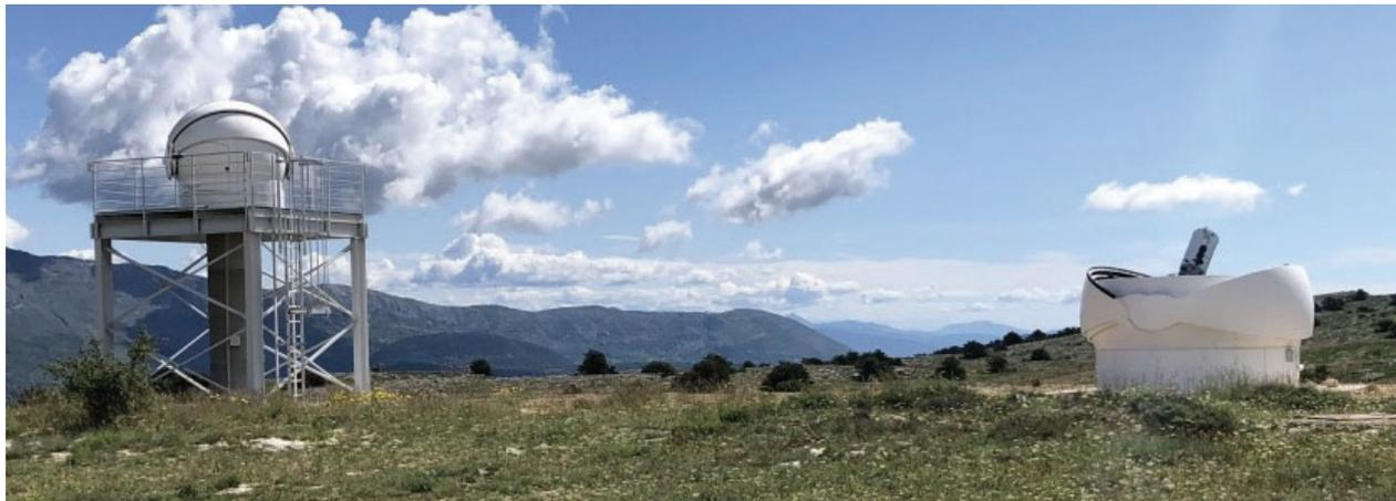
Figure 1. CATS station installed on the Calern Observatory. The left instrument is the G-DIMM, and the right one is the PML.
