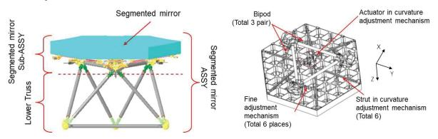
Figure 2. the configuration of the full-scale model. (left): The Segmented mirror ASSY; (right): The Segmented mirror Sub-ASSY. The segmented mirror ASSY includes the segmented mirror Sub-ASSY and lower truss. The segmented mirror Sub-ASSY consists of a segmented mirror, bipods, 6-axes adjustment mechanisms, and curvature adjustment mechanisms.
