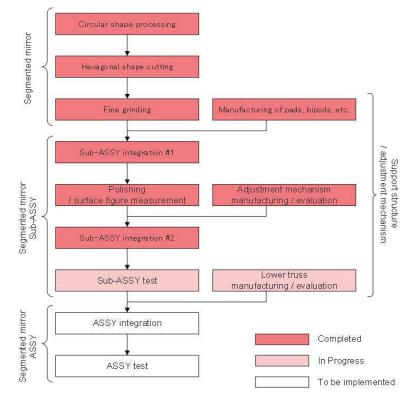
Figure 5. The outline of the manufacturing and evaluation plan for this prototype.
