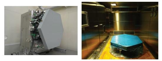
Figure 10. The Sub-ASSY test configuration. (left): 6-axes adjustment mechanism operation test. (right): Thermal cycle test.
