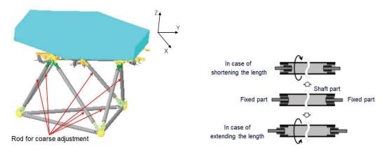
Figure 4. The coarse adjustment mechanisms in the six rods on the lower truss (left). A schematic diagram of rod length adjustment (right).
