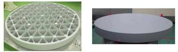
Figure 6. Appearance of the segmented mirror at the stage of "circular shape processing". (left): stage prior to ceramic sintering (after lightweight processing). (right): stage when the "circular shape processing" was completed.
