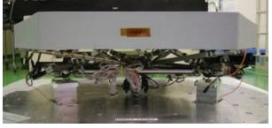
Figure 9. The segmented mirror Sub-ASSY after polishing. (left): Appearance of after polishing (the configuration of the surface figure measurement). (right): side view with the 6-axes adjustment mechanisms and the curvature adjustment mechanisms after Sub-ASSY integration #2.
