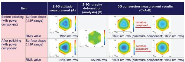
Table 6. Segmented mirror Sub-ASSY absolute surface shape measurement results (before and after polishing).
