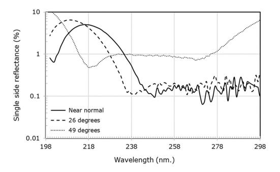
Fig. 1. Spectral performance of a multilayer Al<sub>2</sub>O<sub>3</sub>/MgF<sub>2</sub> AR coating optimized for a wide angle of incidence.
