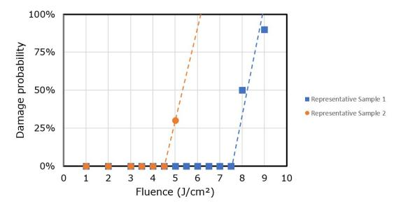
Fig. 3. LDT results for multilayered Al<sub>2</sub>O<sub>3</sub>/ MgF<sub>2</sub> coatings at 248 nm.
