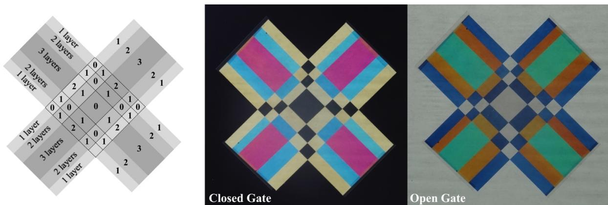
**Fig. 3.** Clear birefringent gift-basket wrap layered and viewed between two polarizers. This six-layer arrangement provides a demonstration of additive and subtractive birefringence, wherein layers oriented in parallel add and layers oriented at 90 subtract. The Closed Gate arrangement (middle panel) is placed between crossed-polarizers. In the Open Gate arrangement, the two polarizers are aligned with parallel polarizations.
