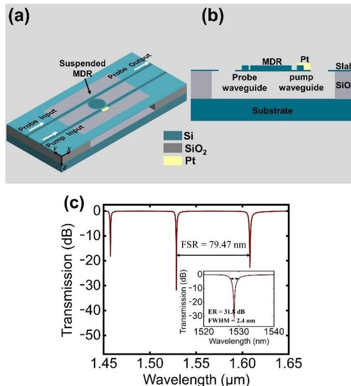
Figure 1. (a) 3D view and (b) yz cross-section of the all-optically tunable filter based on a suspended silicon MDR. (c) Simulated transmission spectrum of the suspended MDR. Inset: the transmission spectrum around the resonance of 1528.66 nm.
