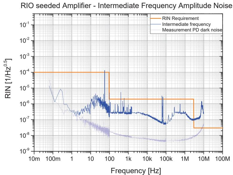
Figure 15 : Power stability intermediate frequency measured with CSEM LH BB with RIO seed laser
