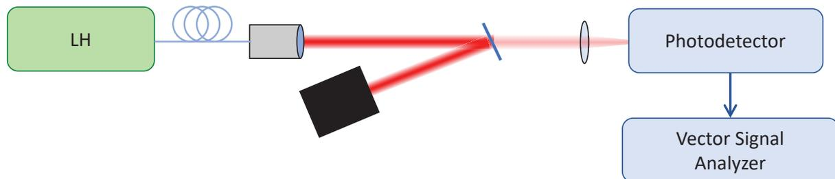
Figure 14 : Intermediate frequency power stability test bench.
