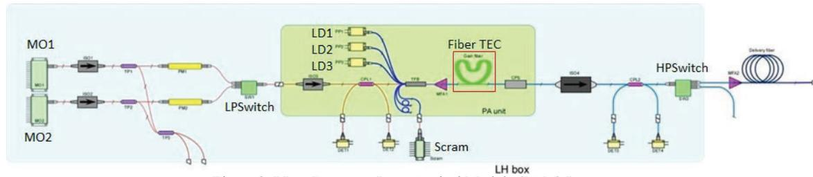
Figure 2: LISA Prototype Laser Optical Module (LOM) Layout
