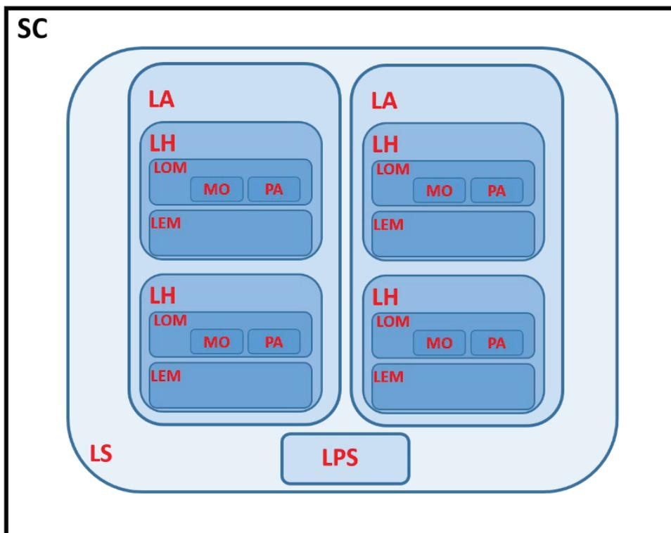
Figure 1: LISA Laser System schematic. SC = Spacecraft, LS = Laser System. LA = Laser Assembly, LH = Laser Head, LOM = Laser Optical Module, LEM = Laser Electronics Module, MO = Master Oscillator, PA = Power Amplifier, LPS = Laser Prestabilisation System.
