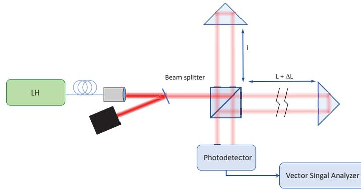
Figure 9: Michelson interferometer for frequency noise measurement in the [3 kHz; 10 MHz] range.
