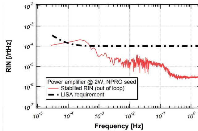
Figure 13: Measurement of power stability with out of loop detector
