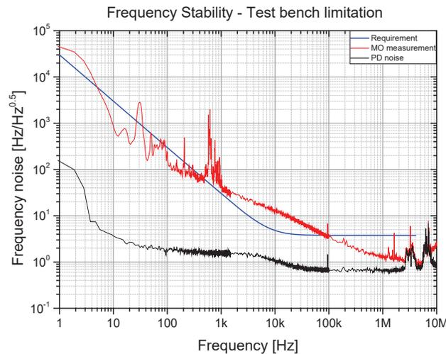
Figure 10: Blue curve represent the high frequency, frequency noise requirement. The red line is the measurement realized on a MO laser (OE-waves). The black curve represents the dark noise of the photodetector.
