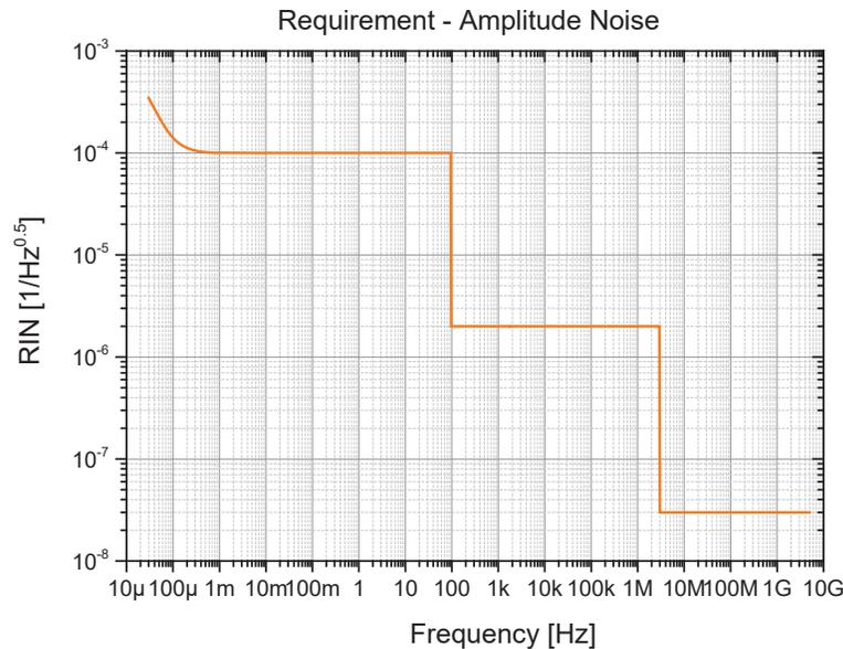
Figure 11 : Output power stability RIN from the development requirement specification in orange
