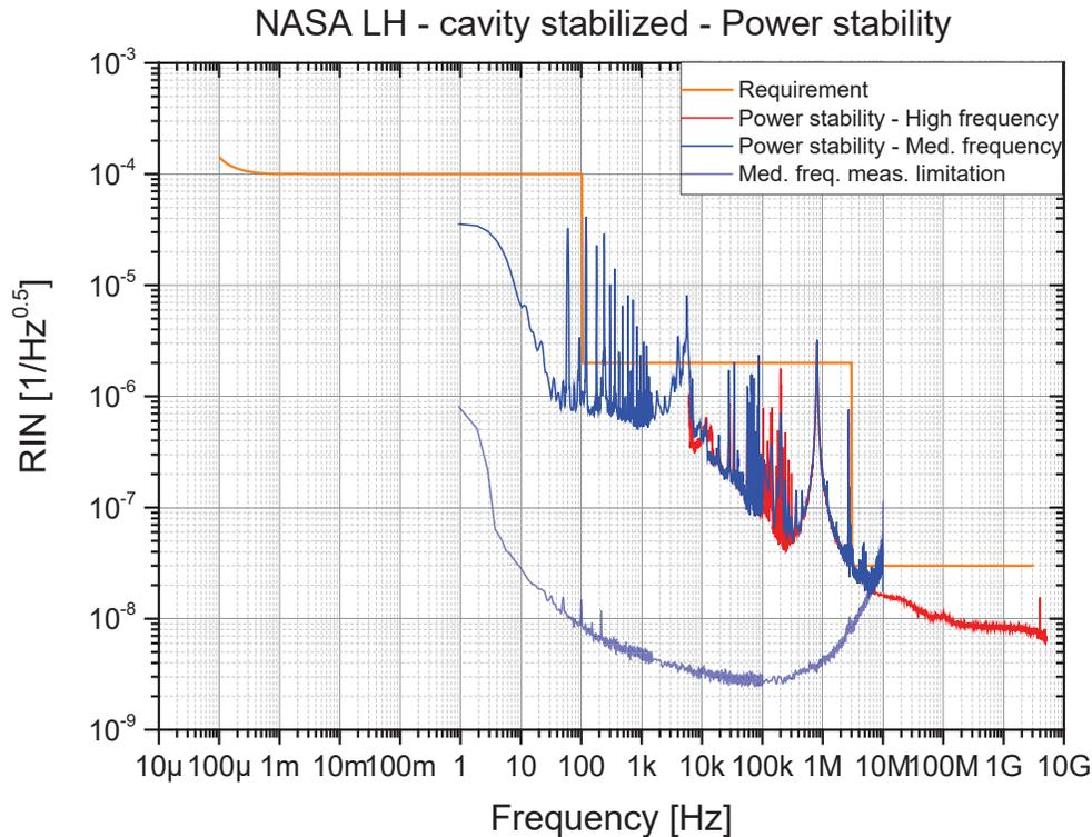
Figure 21: NASA LH cavity stabilized power stability measurement (blue / red curve). The blue curves represent the intermediate frequency range measurement performed with a counter with a vector signal analyser. The red curve is the high frequency range measurement performed with a signal analyser.
