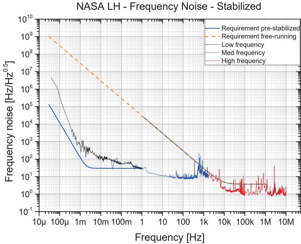
Figure 20: NASA LH cavity stabilized frequency noise measurement (black / blue / red curve). The black and blue curves represent the low and intermediate frequency range measurement performed with a counter with two different gate times. The red curve is the high frequency range measurement performed with the interferometer.
