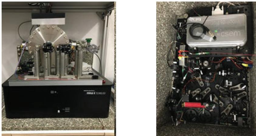
Figure 8: CSEM reference cavity and frequency comb
