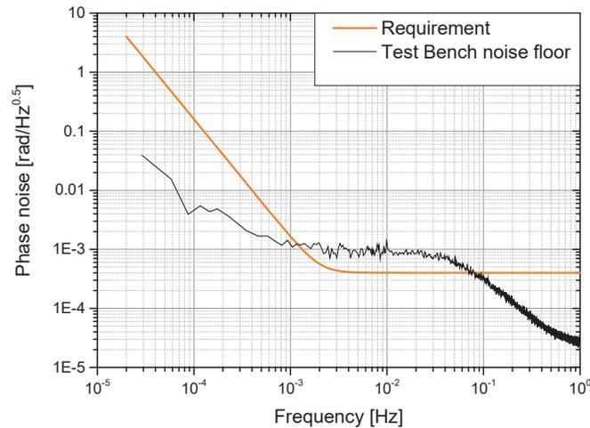
Figure 5 : Sideband phase noise test bench noise floor
