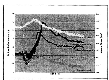
Figure 5 a: Plot of biophysical measurements recorded during sequential laser exposures. The changes in diffuse reflectance  $\Delta I(t)$  (arbitrary units) and internal stress  $\Delta\sigma(t)$  (arbitrary units) from baseline values are plotted.
