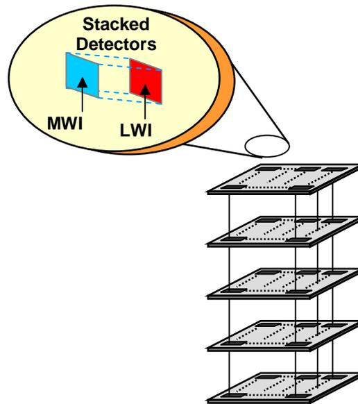
Figure 1 Vertically Integrated Sensor Architecture with multiple levels of signal processing at the detector
