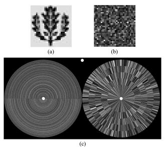
Fig. 6. Example of distortion-invariant ID tag built from an encrypted signature with a large number of pixels. (a) Original signature f(x,y); (b) Encrypted signature  $\psi(x,y)$ ; and (c) Distortion-invariant ID tags. The information of the optical code in the scale-invariant tag is distributed in concentric circles.
