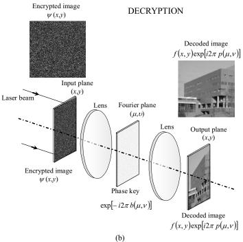
Fig. 2. Optical setup for double phase: a) encryption and b) decryption.
