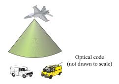
Fig. 1. Example of a distortion-invariant passive optical ID tag.
