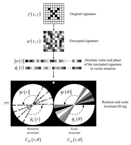
Fig. 4. Synthesis of a distortion (rotation and scale)-invariant ID tag.
