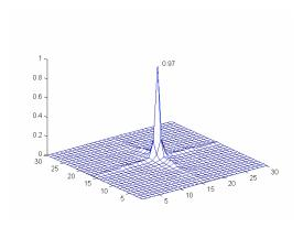
Fig. 8. Normalized output plane for the decoded signature obtained from a rotated version (80 degrees) of the ID tag (Fig. 6c). Parameter k=0.5 is used.
