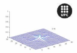
Fig. 13. Decoding a different signature with the correct phase key. The ID tag was rotated 40 degrees and scaled by a factor of 0.6. Correlation output for k=0.5 when the decoded image is compared with the stored reference image (Fig. 6a).
