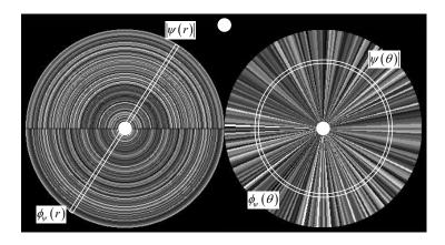
Fig. 5. Rotation and scale invariant recovering the encrypted signature from the optical code of the ID tags of Fig.4.
