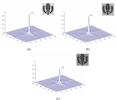
Fig. 11. Decoded signatures and correlation outputs (k=0.5) for simultaneously rotated and scaled versions of the ID tag shown in Fig. 6c. (a) Scale factor: x 0.6 and rotation angle: 40°; (b) Scale factor: x 0.5 and rotation angle: 60°; (c) Scale factor: x 0.4 and rotation angle: 70°.
