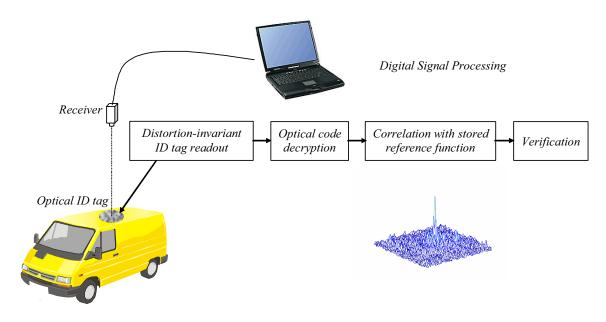
Fig. 3. Block-diagram of the remote identification system.
