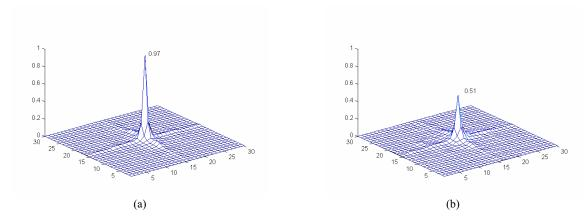
Fig. 10. Normalized output planes for the decoded signatures obtained from rotated version of the ID tag (Fig. 6c). Parameter k=0.5 is used. The ID tag was scaled by a factor (a) 0.4, and (b) 0.2.
