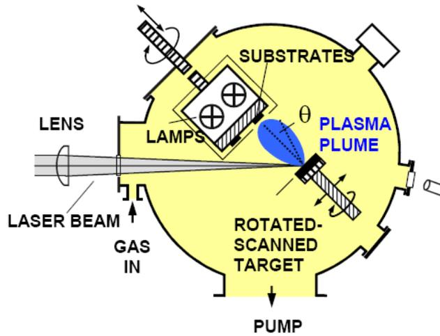
Figure 1. Schematic of experimental setup for pulsed-laser deposition of thin films in “on-axis” geometry. The distance between target and substrate is several cm, typically.
