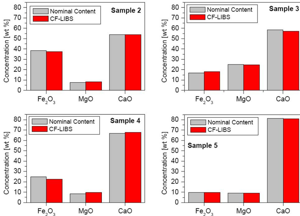
Figure 3. CF-LIBS analysis of four samples containing different amount of iron oxide, magnesium oxide, and calcium oxide. Oxide concentration as determined by CF-LIBS (red columns) and nominal concentration (grey columns).
