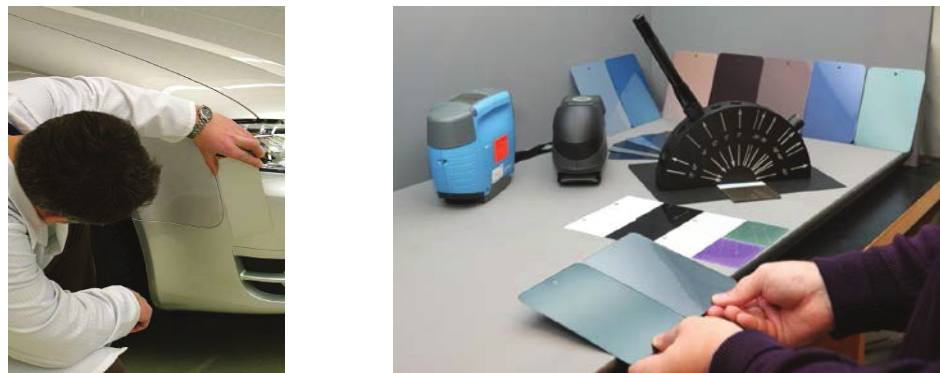
Figure 5. Example of a bad color harmony in the frontal side of a car (left); visual comparison in color, gloss and texture of a sample pair inside a diffuse lighting booth (right), with some color devices (from left to right: multi-angle spectrophotometers BYK-mac, X-Rite MA98 and gonio-vision-box).
