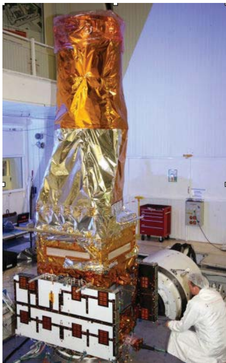
Fig 12 Instrument mounted on Proteus platform
