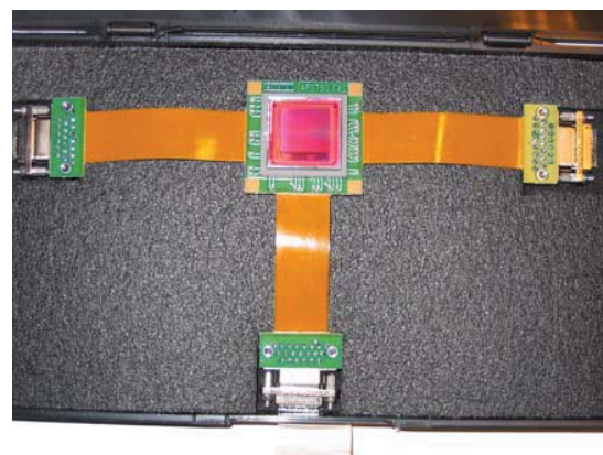
Fig. 3: CIS acquisition and tracking sensor developed by EADS Astrium and Supaéro/CIMI for optical communication
