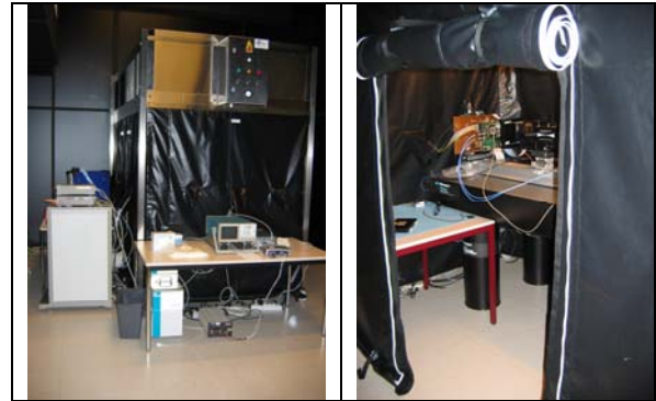
Fig. 2-11: COBRA2M FM test bench in clean room with class 100 flux and device regulated at 17°C.
